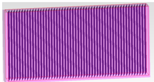
Figure 40 Vertical arrangement of louver blades
