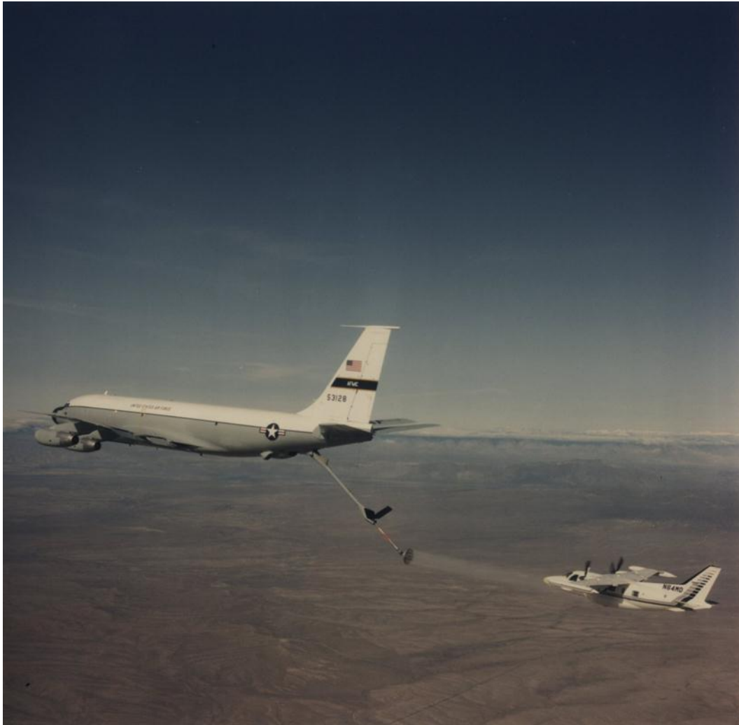
Figure 1. United States Air Force Icing Tanker SN 55-3128 in formation with the Mitsubishi MU-2B-60 test aircraft in the water stream.
