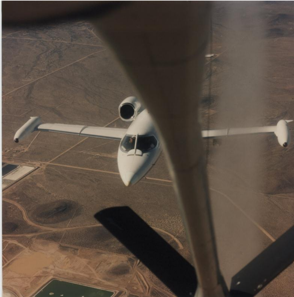
Figure 2. Gates Learjet Model 36 chase aircraft during a calibration sweep of the cloud being emitted from the icing tanker nozzle.
