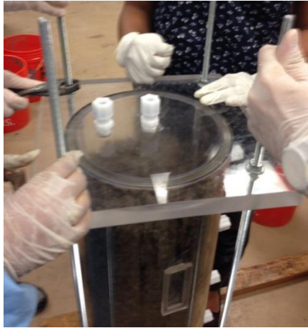
Figure 3-12 Sealing the column with top sealing plate
