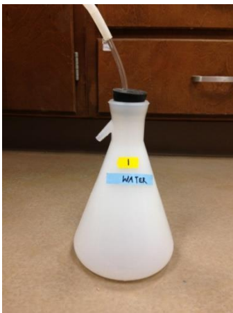
Figure 3-7 Humidifier set up
