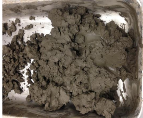
Figure 3-11 Mixture of fly ash, soil and water
