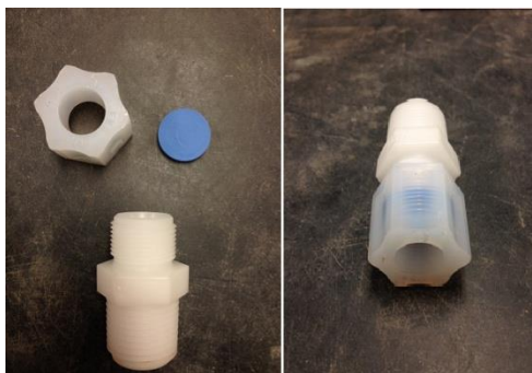
Figure 3-8 Compressions fittings for methane port (left) and assembled methane port (right)
