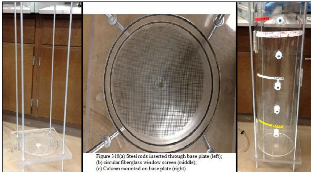
Figure 3-10 (a) Steel rods inserted through base plate (left); (b) Circular fiberglass window screen (middle); (c) Column mounted on base plate (right)
