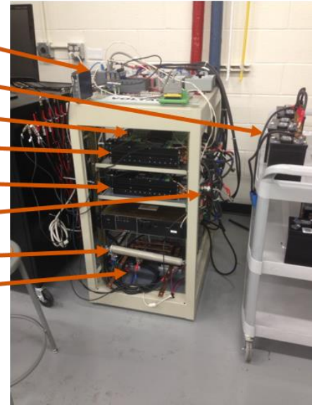
Figure 28: Experimental setup of the bi-directional test of a COTS HESM [25]
