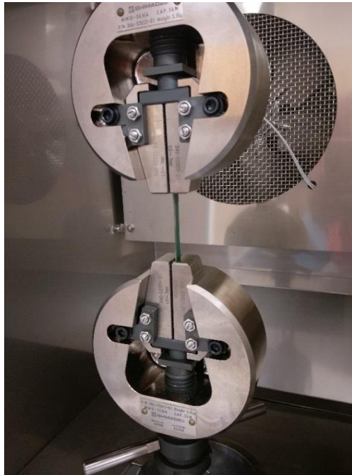
Figure 4.7: Samples inside the Jaws of Shimadzu
