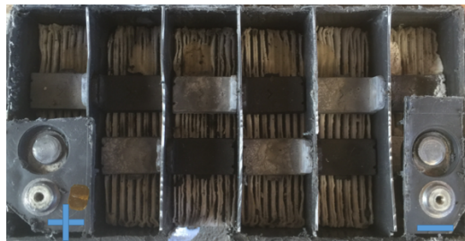
Figure 4-25. UPS400MR disassembled to show inner configuration of cells and bus work.
