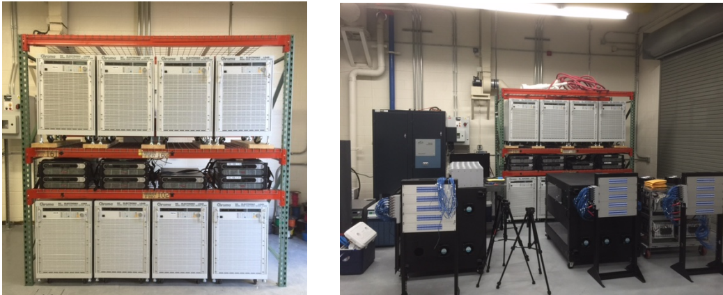
Figure 3-6. Photograph of eight of nine 15 kW programmable loads and eight 15 kW power supplies used in this research. In the left most figure, a zoomed in view of the loads and supplies is shown. In the right most figure, the full setup is shown.
