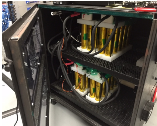
Figure 3-12. Photograph of the 20S/2P Saft LFP-LI battery assembled in a test chamber. As they are shown, they are housed in plastic housings used for evaluation with forced-air cooling.
