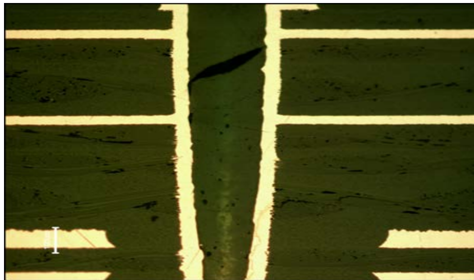
Figure 5: Cross section of PCB plated through-hole on oil exposed server [21]
