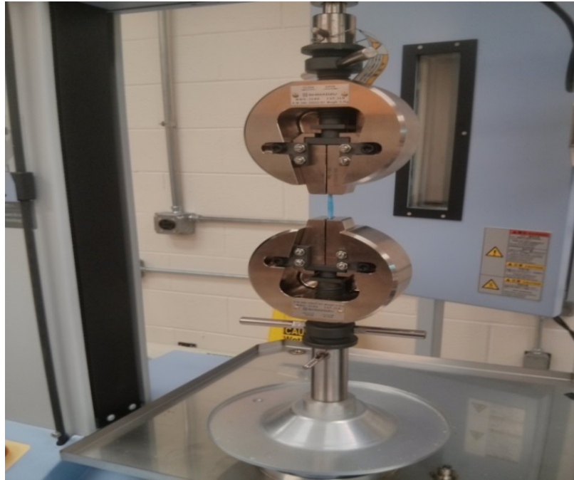
Figure 10: Test setup to measure mechanical properties of cable specimen
