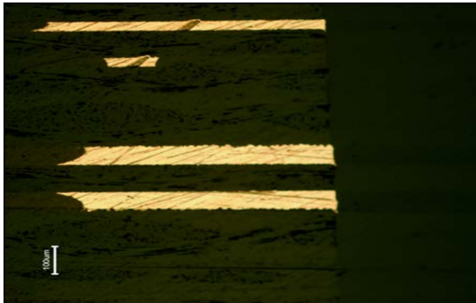
Figure 6: Edge of oil exposed PCBs maintain structural integrity and show no indication of delaminating [21]
