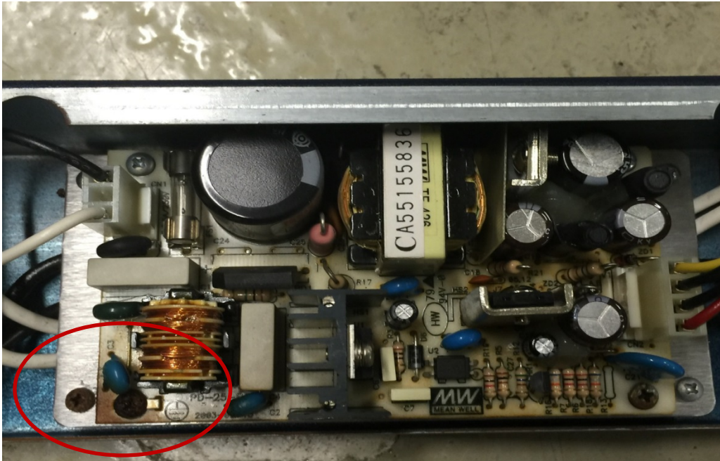
Figure 3: Rust on the mounting screw
