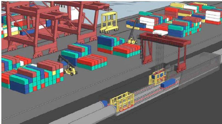
Figure 1-1 Schematic of a UFT System (Winkelmans, 2009)
