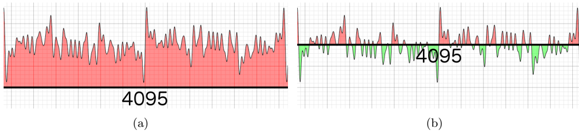
Figure 5.8. A representation of (a) fully saturated values and (b) partially saturated values in a 12-bit sampler.
