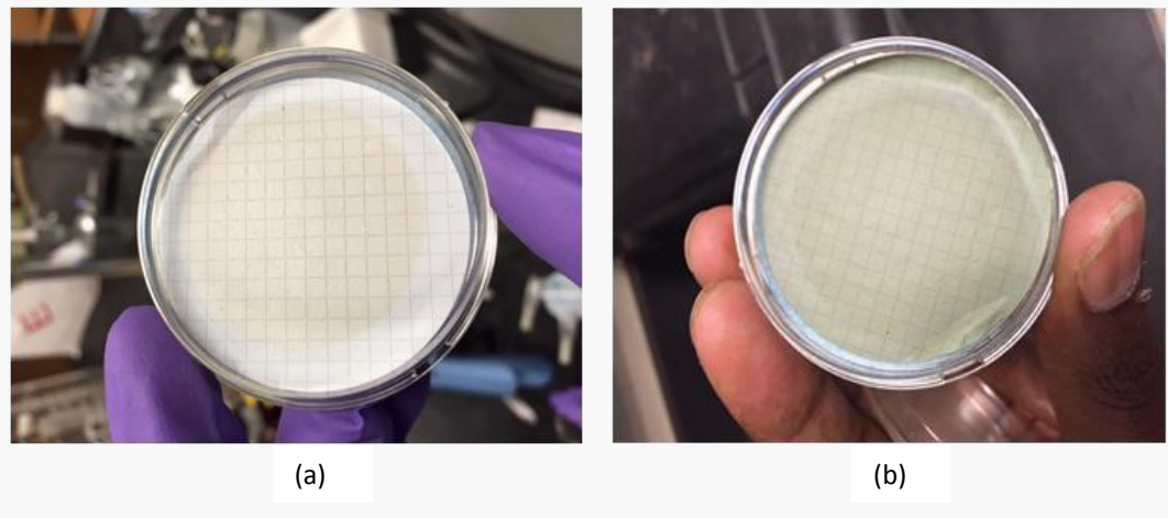
Figure 4.17 Petri dish with filtered sample (a) before incubation, (b) after incubation
