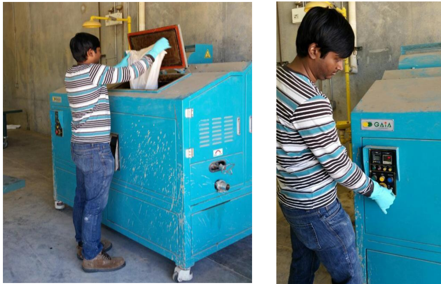
Figure 3.11 GAIA food waste dryer loading and operation
