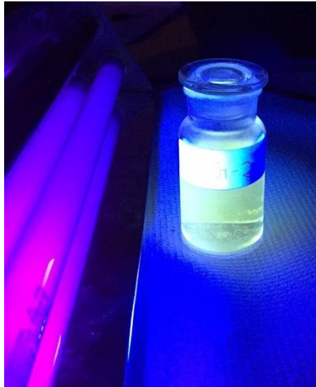
Figure 4.16 Non-fluorescence of sample G-2 indicating absence of enterococci in the sample
