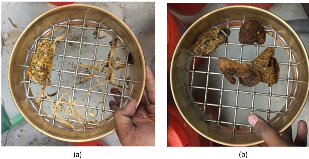
Figure 4.10 Portion of grocery samples retained on 1" sieve (a) Corn cobs, (b) fruit peels
