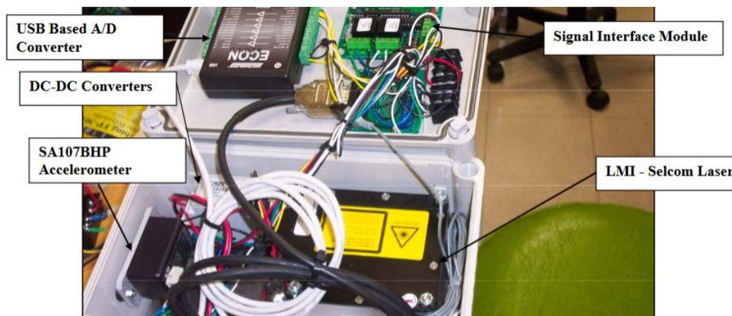
Fig 1.1 A laser based road profiler. [10]
