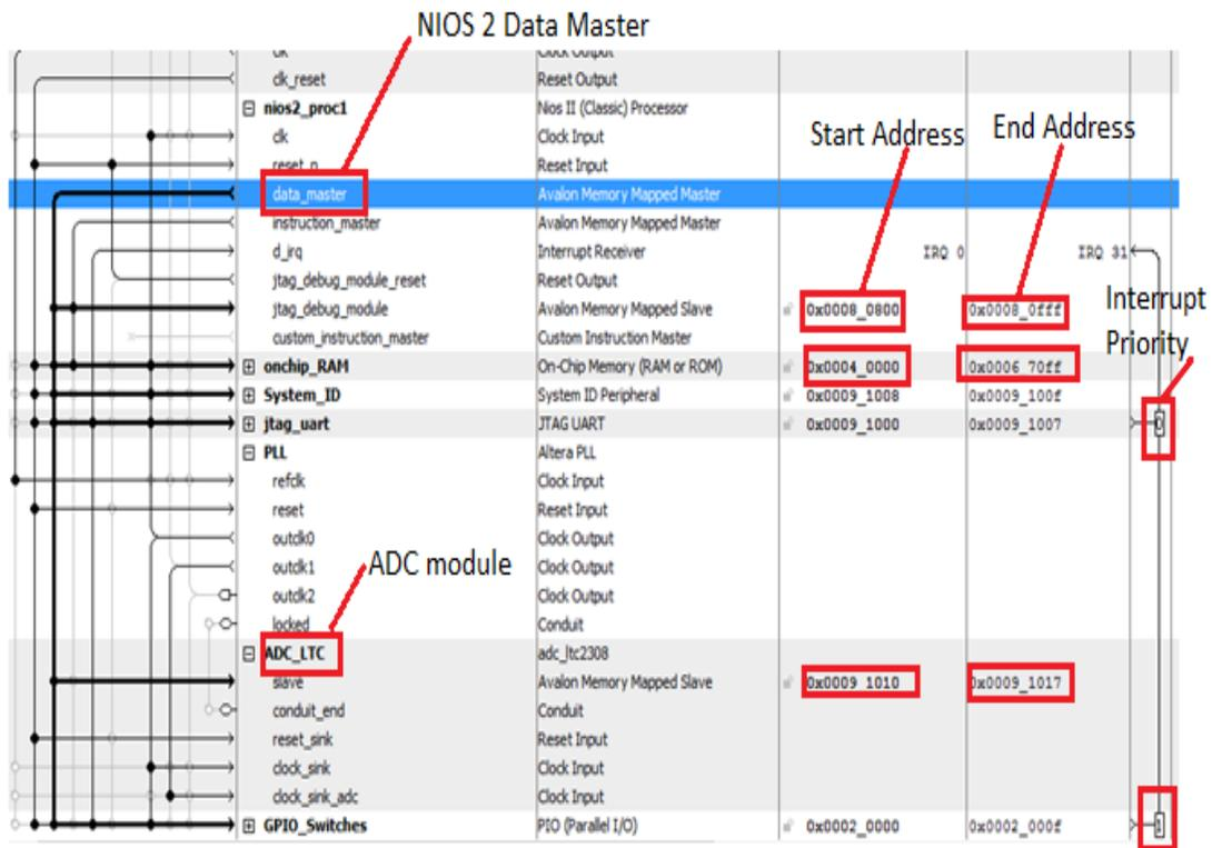
Figure 5.2 QSYS snapshot for FPGA fabric interconnect.
