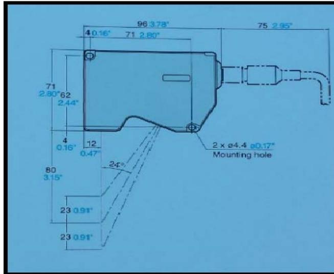
Figure 3.20 Keyence LJ - V7080 sensor head dimensions and measurement range. [19]
