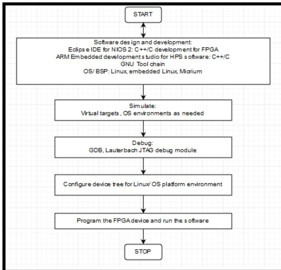
Figure 4.3 Software design flow diagram for DE1 SOC FPGA board
