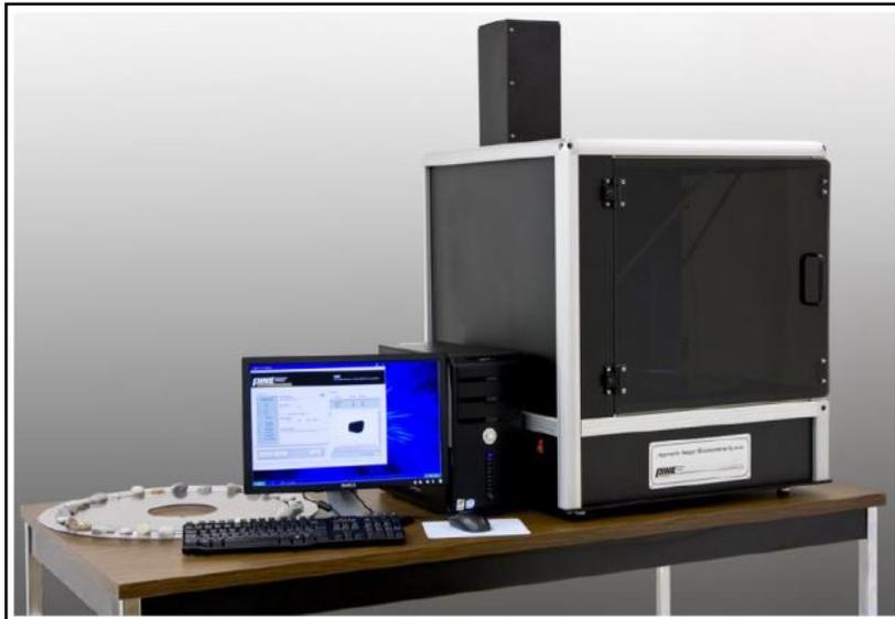
Figure 1.4 AIMS, Aggregate Imaging Measurement System. [13]
