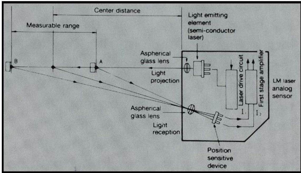
Figure 3.1 Laser triangulation technique for NAIS LM 200 Laser sensor [5]
