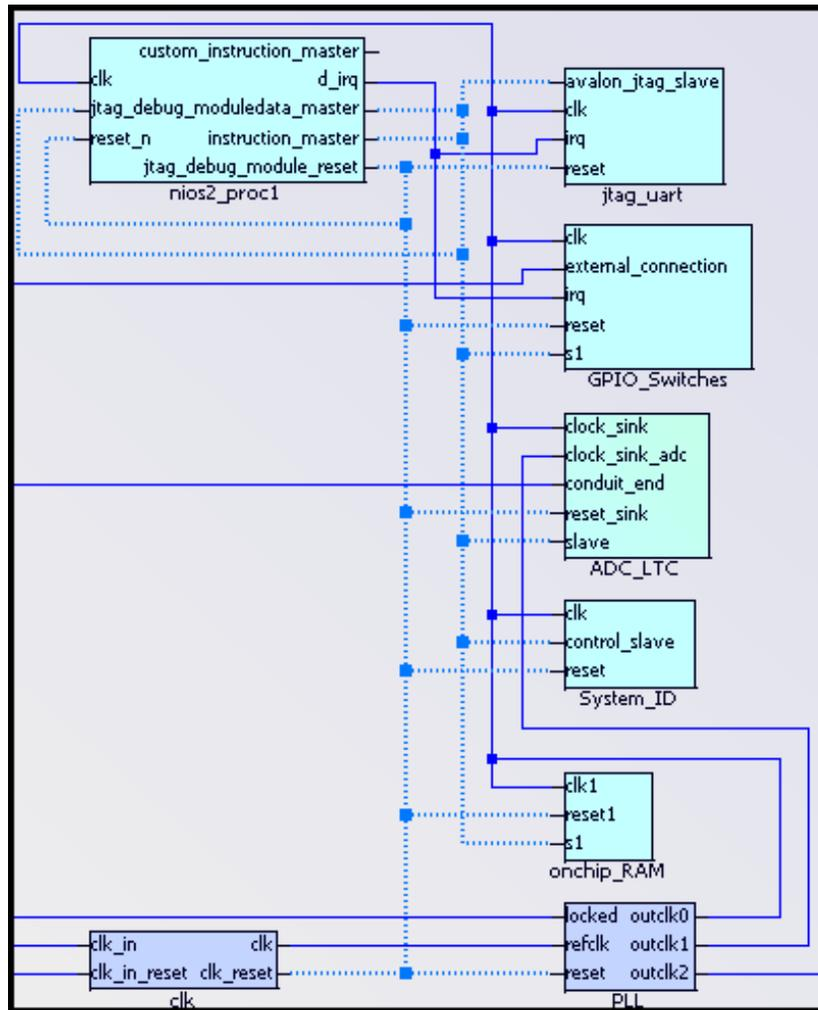
Figure 5.5 FPGA configuration schematic for basic ADC functionality
