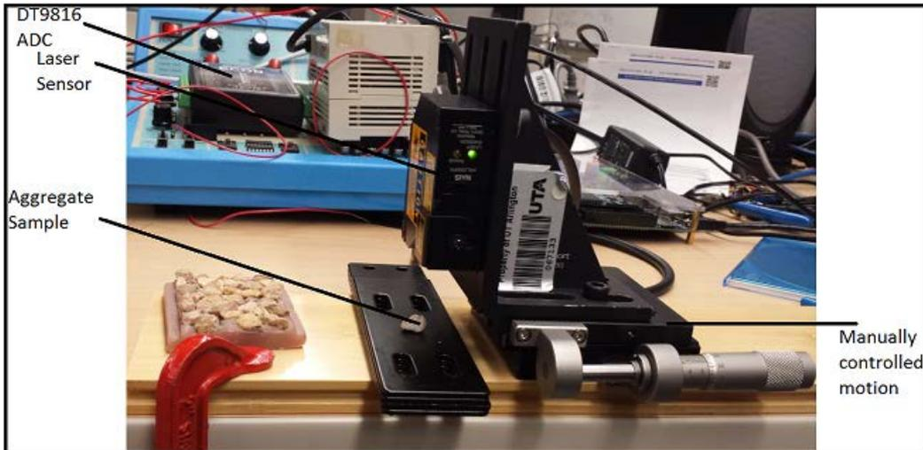
Figure 3.12 Laboratory setup for test equipment.
