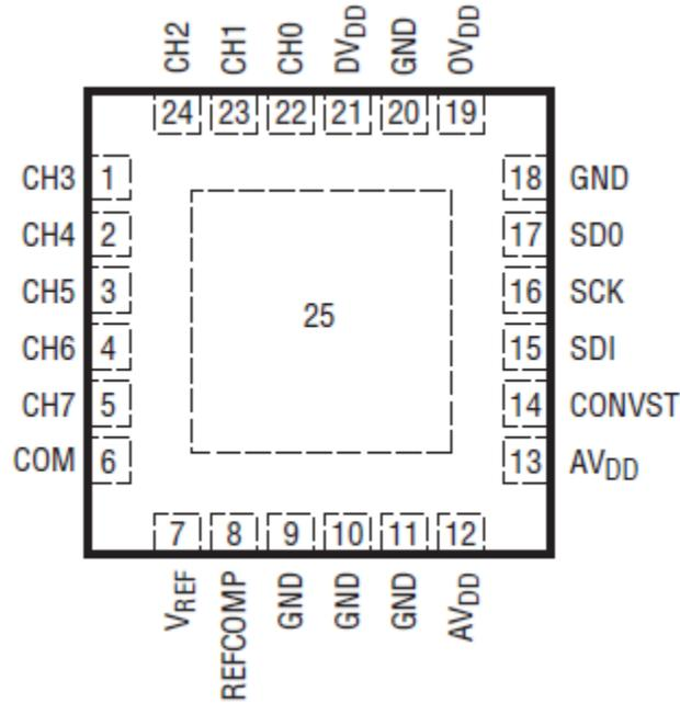
Figure 5.10 Pin diagram of Linear Technology LTC 2308 ADC converter. [16]
