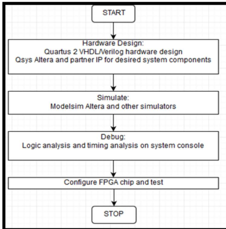
Figure 4.2 Hardware design flow diagram.
