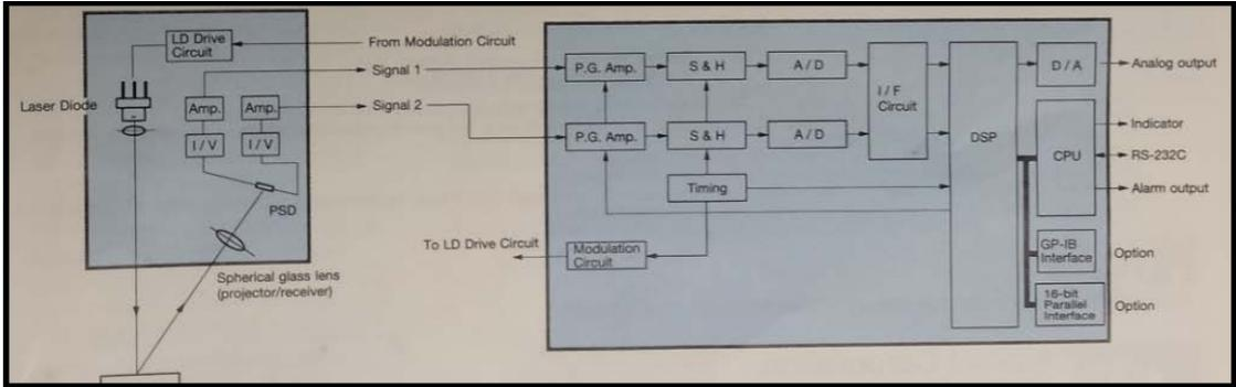
Figure 3.6 NAIS LM 300, inbuilt A/D conversion and measurement system. [20]
