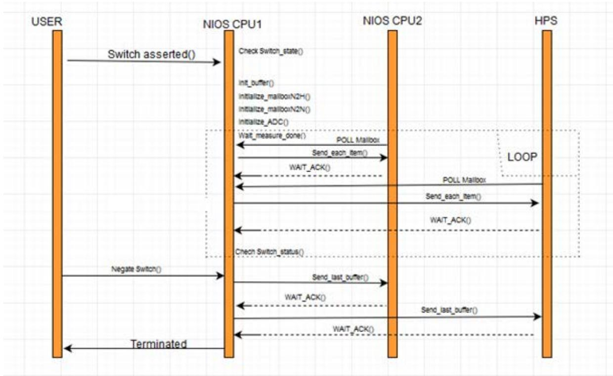
Figure 5.14 Time sequence diagram for FPGA side operations.
