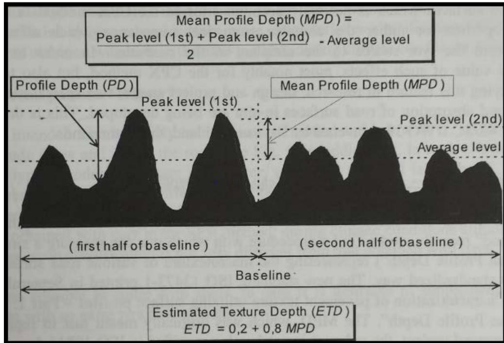
Figure 1.3 Profile Depth and Mean Profile Depth calculations. [12]
