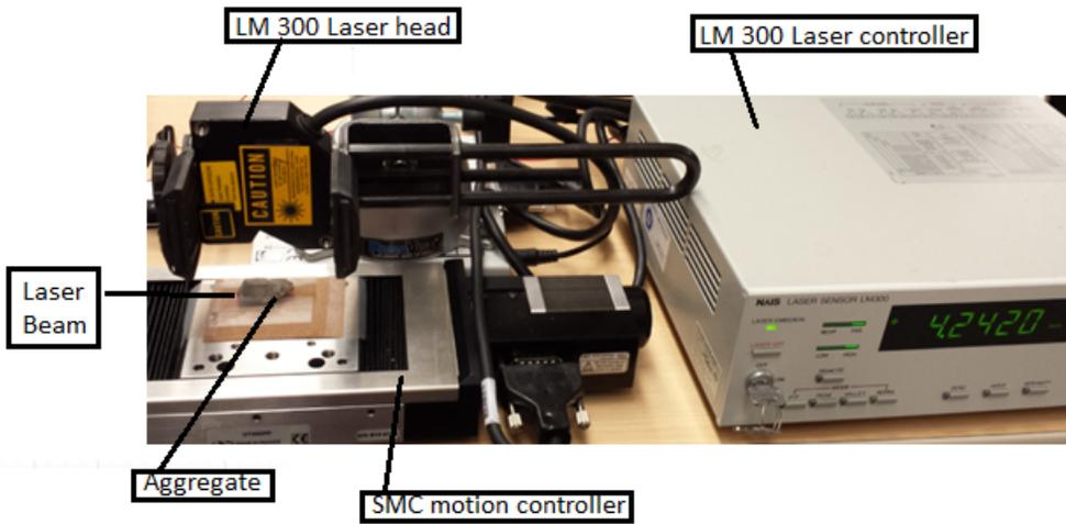
Figure 6.2 LM300 with SMC Motion control system
