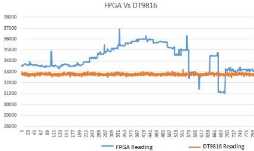
Figure 6.4 Comparison of Level of detail between 800 points obtained from DT9816 board and FPGA board.
