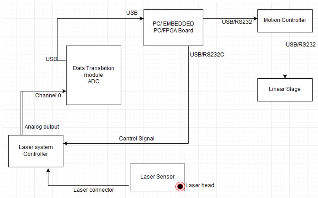
Figure 3.11 Block Diagram of Laser Measurement System and control flow
