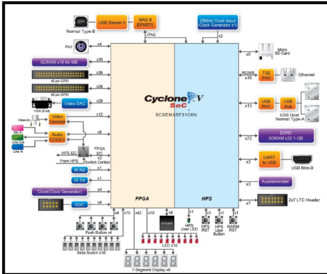
Figure 4.1 BLOCK Diagram of DE1 SOC Board [14]
