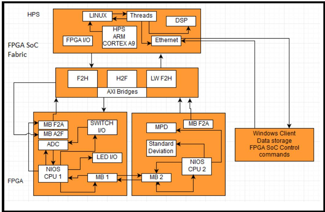
Figure 5.7 Complete Soc architecture for data acquisition, processing and Ethernet communication
