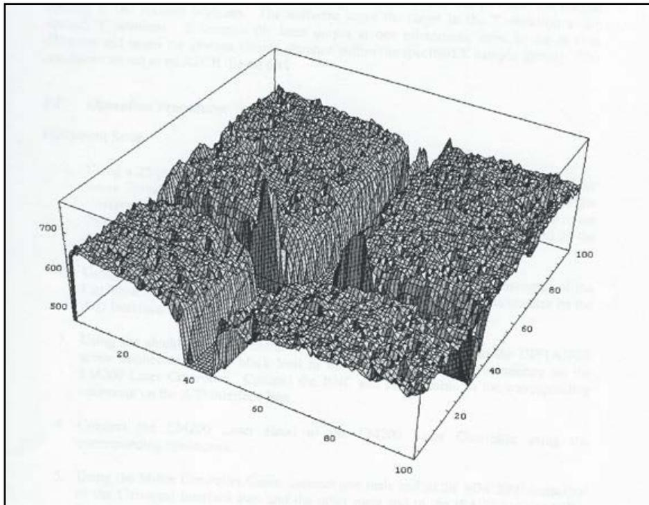
2.2 Figure three dimensional scan of a tile joint at UTA floor. [4]
