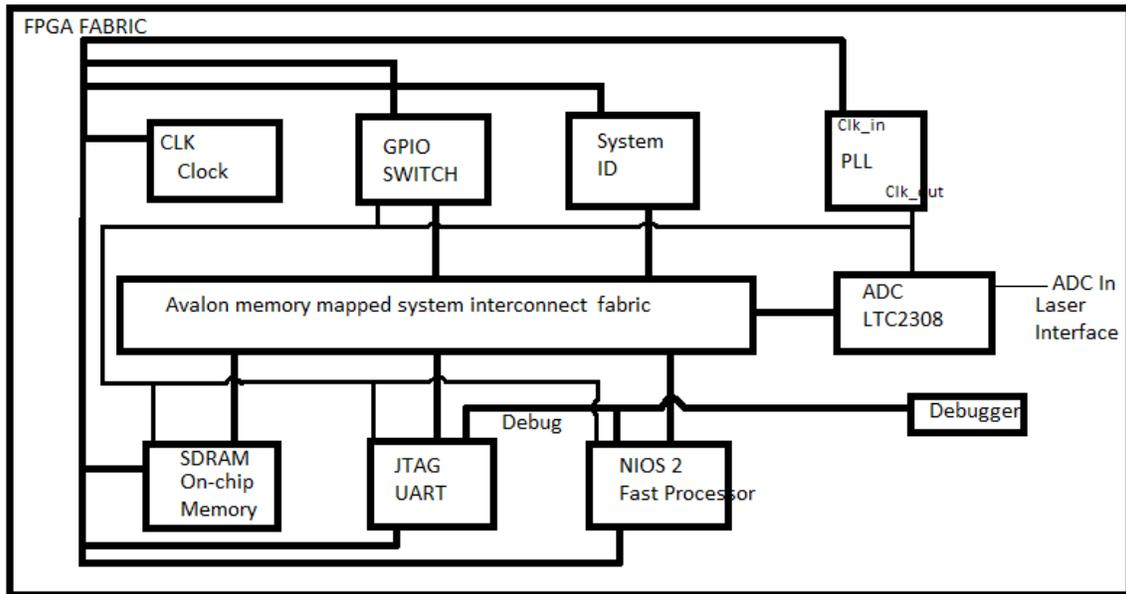
Figure 5.1 Block diagram of ADC data acquisition on FPGA fabric
