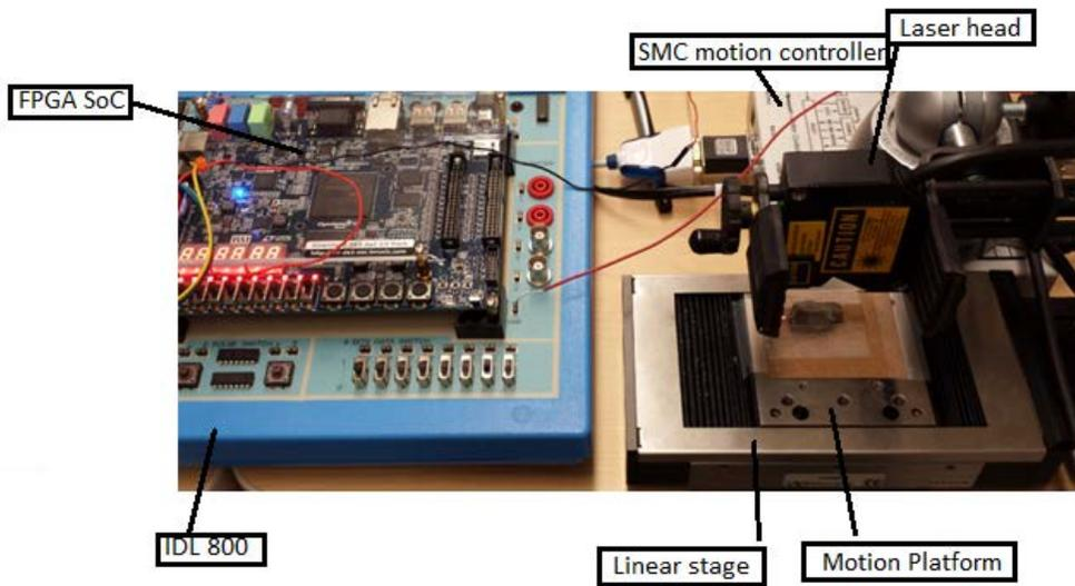
Figure 6.3 Complete FPGA Texture measurement instrument
