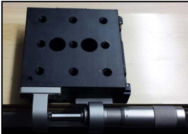
Figure 3.10 manually controlled linear stage, one micrometer step size
