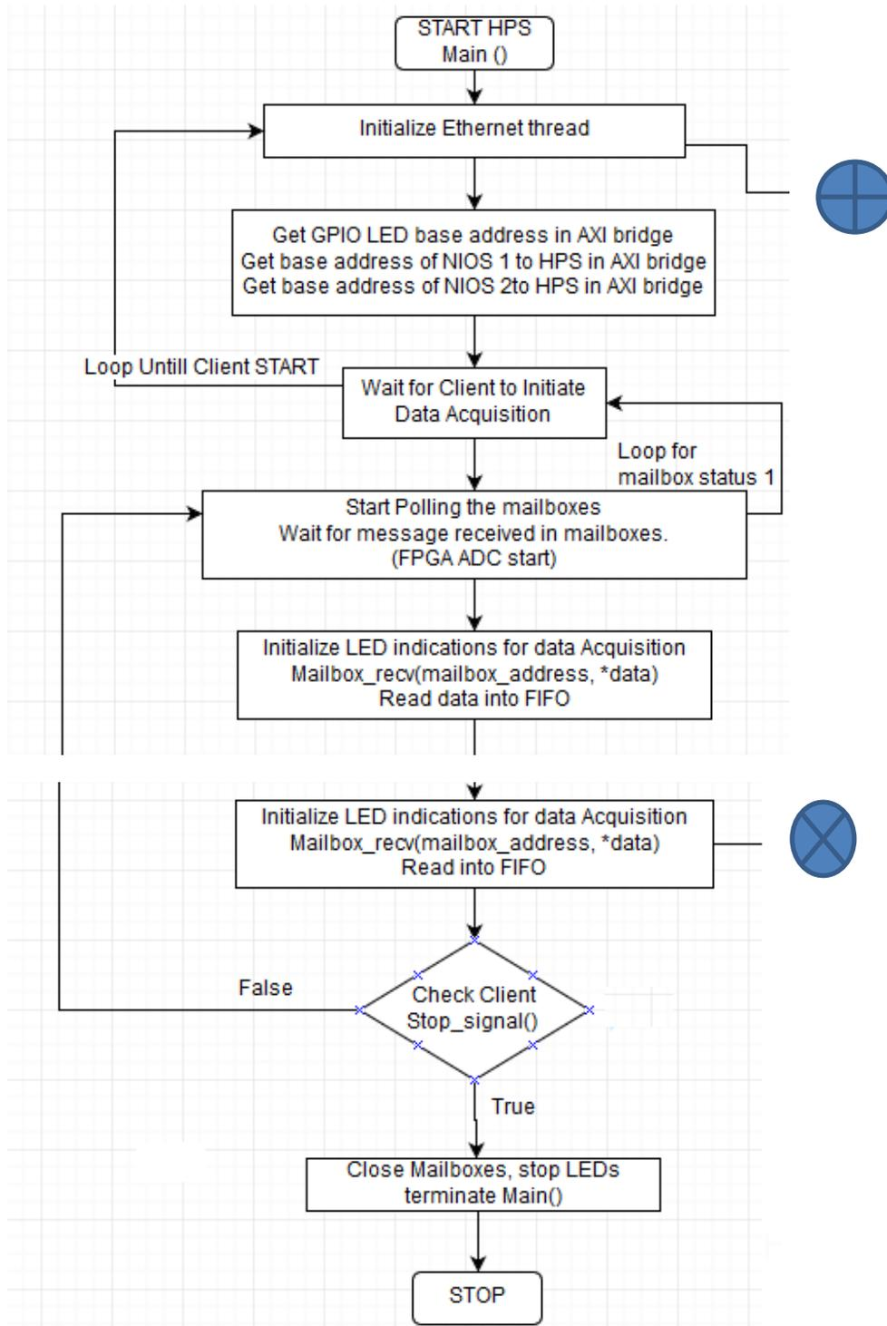
Figure 5.15 Flow chart for HPS multithreaded processing and Ethernet communication.
