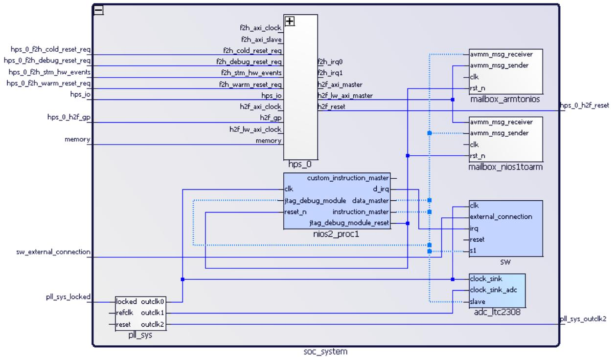
Figure 5.9 Reduced system architecture to illustrate NIOS and HPS connectivity through mailbox cores.
