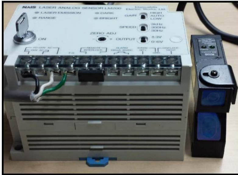
Figure 3.4 NAIS LM 200 Laser sensor and controller
