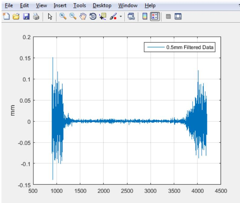
Figure 3.19 Surface estimation using high-pass IIR filter on scanned data.
