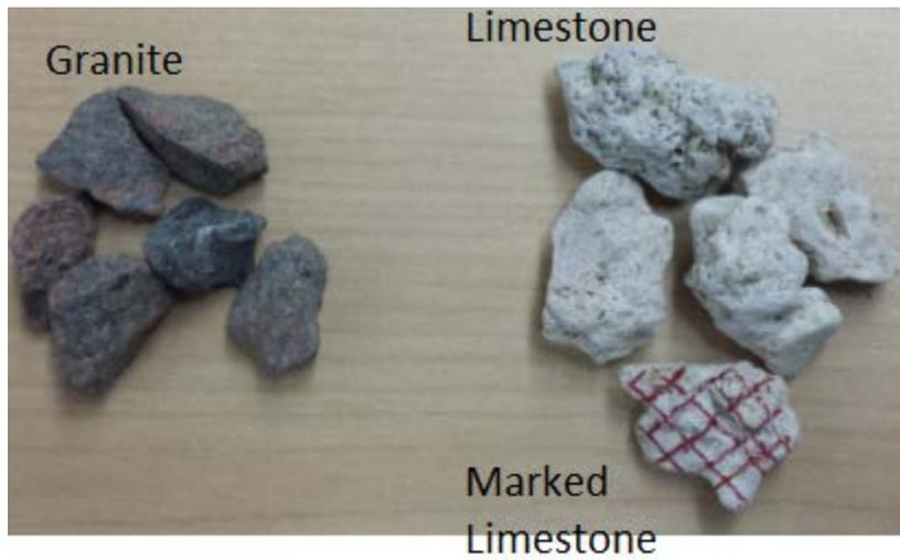
Figure 3.15 Granite, limestone sample and a marked aggregate for analyzing the laser color immunity.
