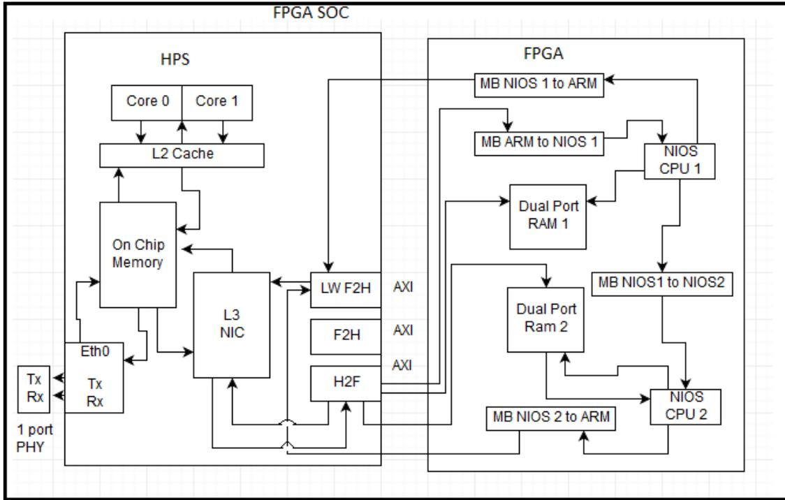
Figure 5.6 Multi-core hardware design and Mailbox inter-processor communication.
