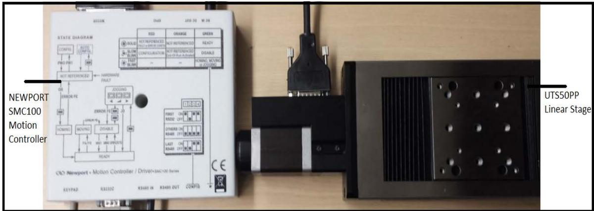
Figure 3.21 Newport SMC100 controller and UTS50PP linear stage
