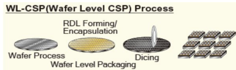
Figure 1-2 Process in Chip Level Package [16]
