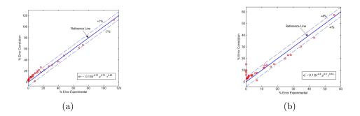
Figure 7.11. Correlations for peak percentage error for infinite plate (a) positive error, (b) negative error.
