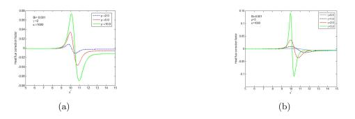
Figure 7.6. Dependence of slot jet infinite plate heat flux corrections on (a)  $\rho$ , (b)  $\gamma \kappa = 1000$  and Bi = 0.001.
