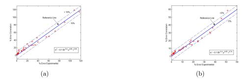
Figure 7.12. Correlations for peak percentage error for finite plate (a) positive error, (b) negative error.
