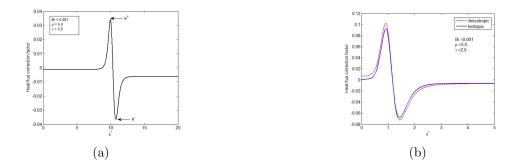
Figure 7.3. (a) Heat flux correction curve illustrating lateral conduction effects for a slot jet over an infinite metal foil. (b) Comparison of finite plate heat flux correction curves for isotropic insulation layer with an orthotropic case, where in-plane thermal conductivity is five times the out-of-plane thermal conductivity.
