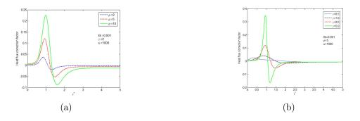
Figure 7.10. Dependence of slot jet finite plate heat flux corrections on (a)  $\rho$ , (b)  $\gamma \kappa = 1000$  and Bi = 0.001.
