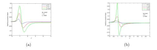
Figure 7.8. Dependence of slot jet finite plate heat flux corrections on (a)  $\rho$ , (b)  $\gamma \kappa = 1000$  and Bi = 0.001.
