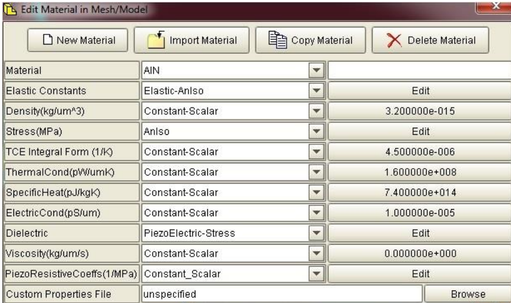
Figure 3.17 Physical Properties of AIN film mentioned in material editor .
