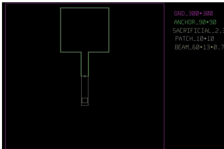
Figure 3.16 2D Layout of the cantilever including bond pad.
