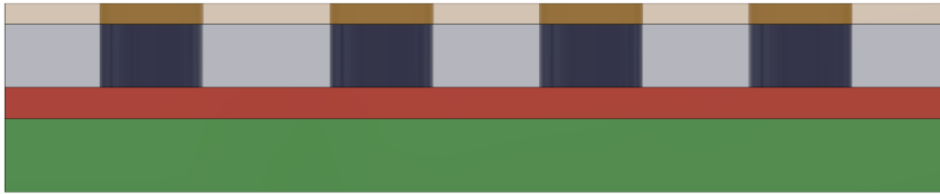
Figure 20 Chrome (50nm) and gold (10nm) deposition
