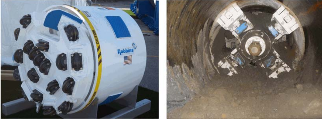
Figure 1-3 SBU cutterhead attachment (left), and a back view of the unit from inside the casing (right) (The Robbins Company, 2016)
