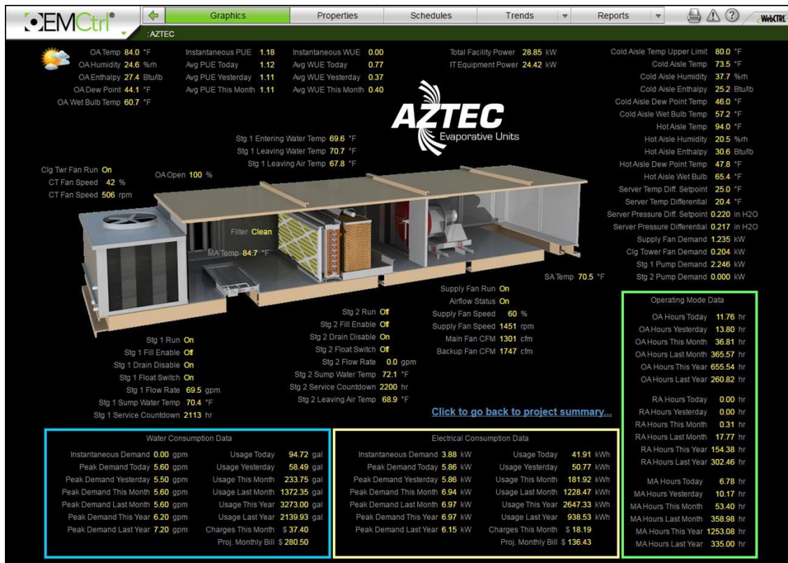
Figure 2.5 Webpage of BAS showing real time data for Research MDC
