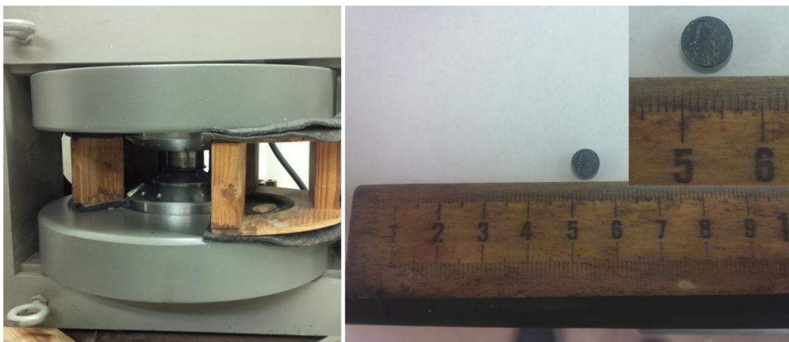
Figure 7.3 Electromagnet used for magnetic alignment (left). Photograph of Co nanowires-epoxy composite sample aligned in 20 kOe field (right).
