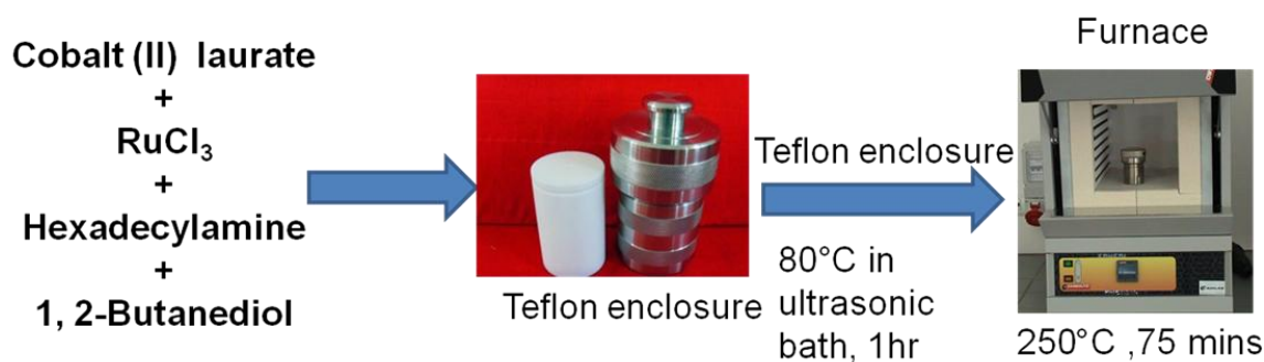
Figure 7.2 Schematic illustration of Co nanowires synthesis process.
