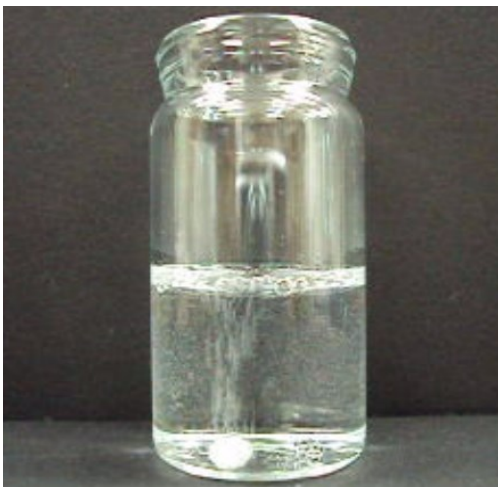
Figure 3-1 Oxygen bubbling Y559(DOPA) KatG-bound glass bead in H_2O_2
