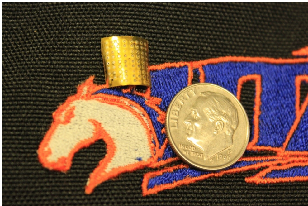
Figure 2-13 1 cm × 1 cm Die of Flexible Substrate Containing 35 Temperature Sensors
