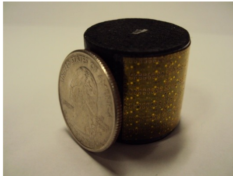
Figure 4-16 A 2 x 2 cm 2 Piece of Flexible Substrate Containing an Array of 75 Pressure Sensors. ©2012 IEEE. Reprinted, with Permission, from MEMS Absolute Pressure Sensors on Flexible Substrate by M. Ahmed, D. P. Butler, Z. Celik-Butler, in IEEE MEMS, 2012 [64]
