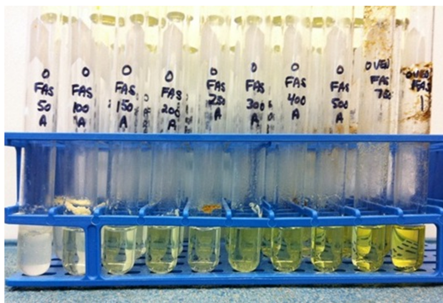
Figure B - 26. Digests using varying amounts of catalyst
