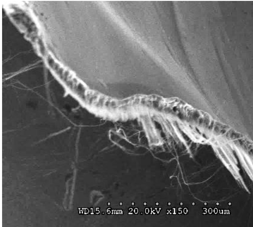
Figure 1 SEM picture of carbon nanotube sheet-collagen composite
