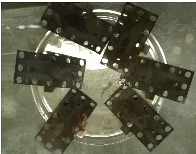
Figure 5.2. Photocathode after the first step and baking for two hours.
