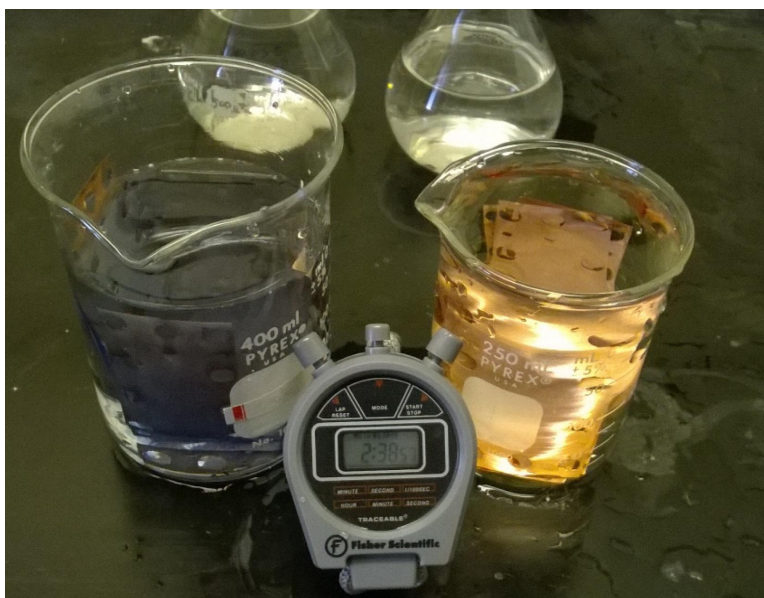
Figure 5.1. Formation of \text{Cu}(\text{OH})_2 on Copper foils after around 2 minutes in the left beaker and fresh copper foil are just inserted in solution in the right beaker.
