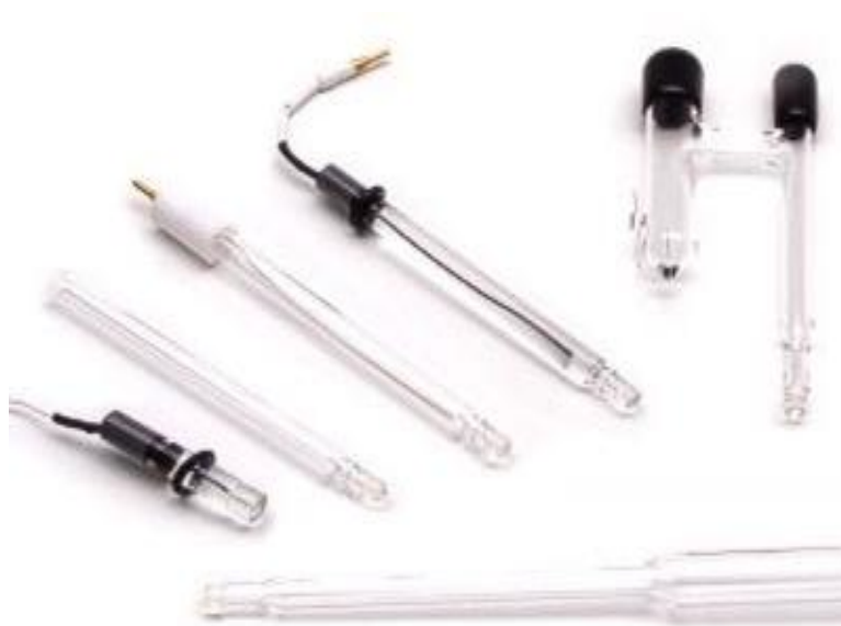
Figure 3.6. Different type of reference electrodes.
