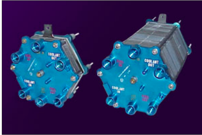
Figure 1.2. Short and Long stacks of PEMFC for different power needs (Image: www.nasa.gov ).
