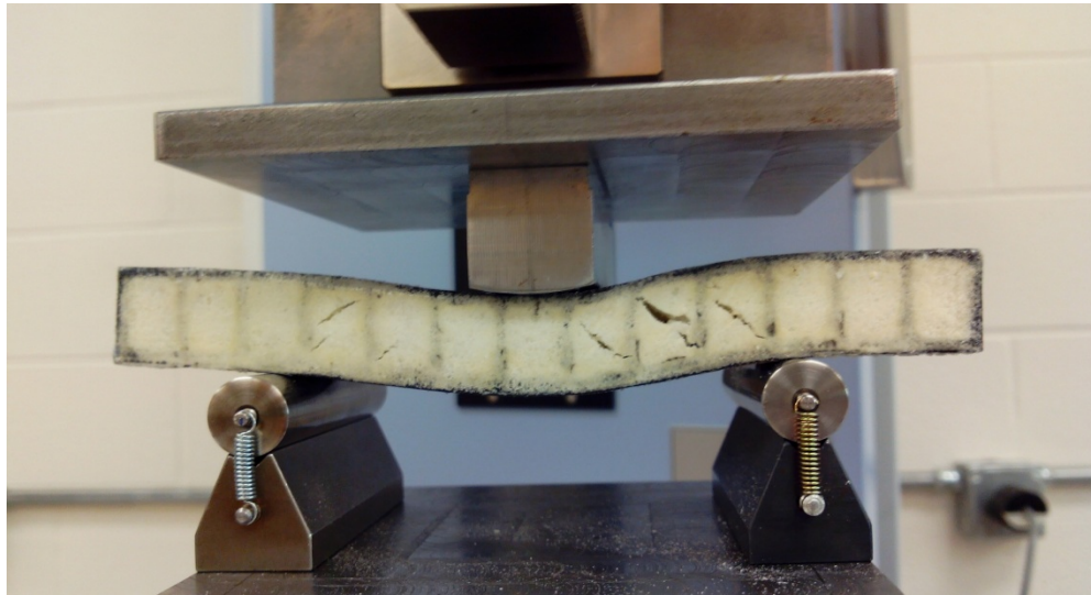
Figure 4-3 Failure of sandwich beam with foam core
