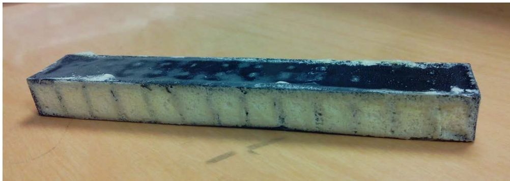
Figure 4-2 Sandwich structure before (a) and after filling with foam (b)
