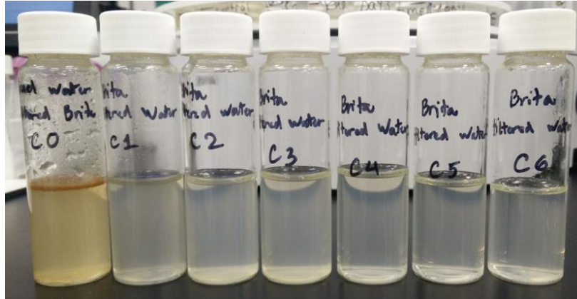
Figure 2-1a. Visible improvement in water quality can be observed after filtering PW5 with Brita filter.
