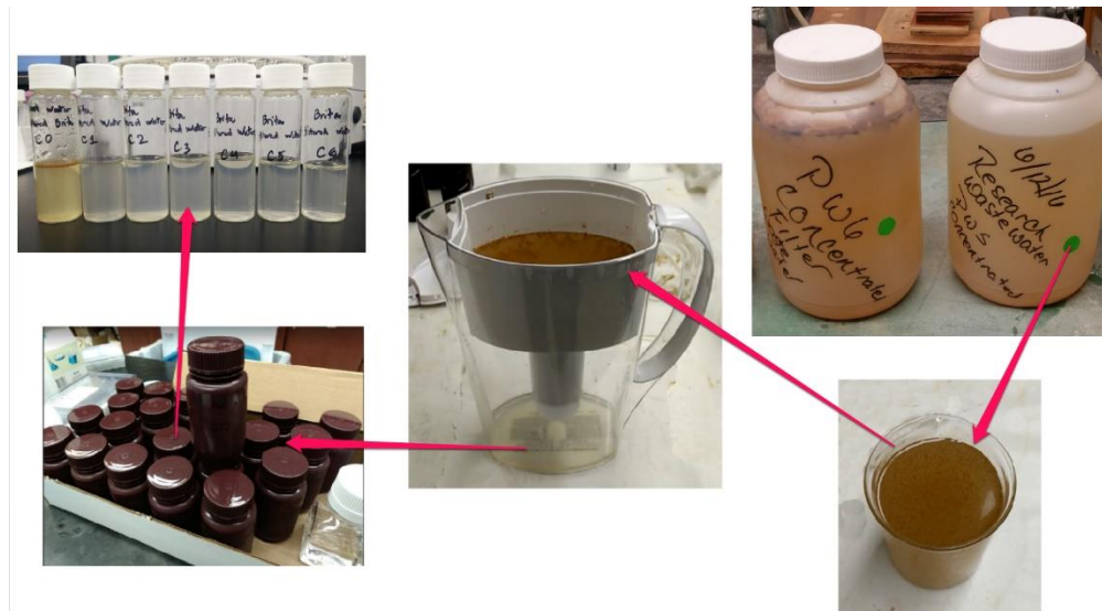
Figure 2-1b. Filtering steps performed on PW sample, each consecutive 130ml eluate collected in brown bottle for further analysis.
