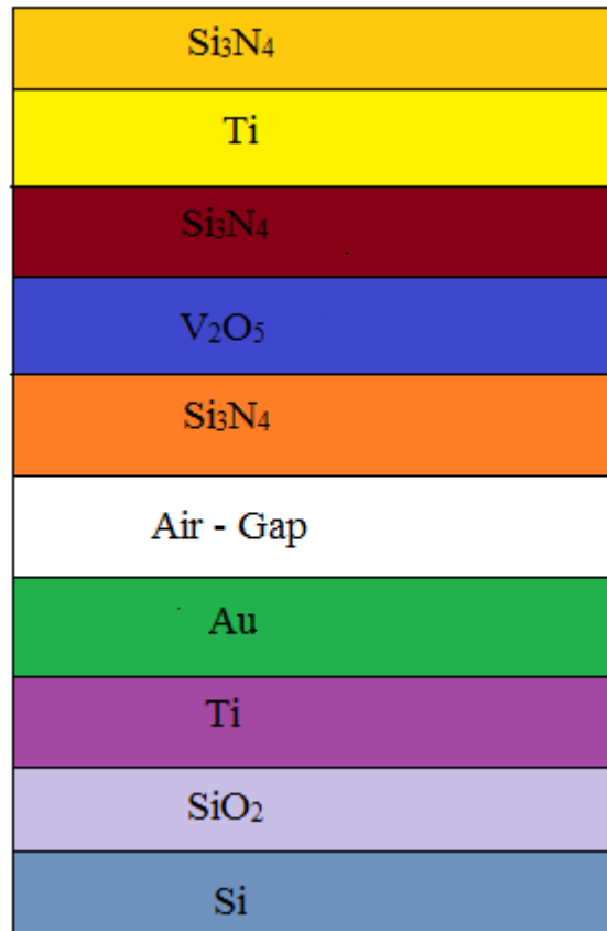
Figure 3-3 Sensor structure proposed by Awad et al. [17]
