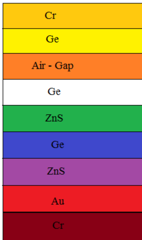
Figure 3-5 Filter structure proposed by Wang et. al. [19]
