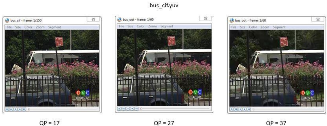
Figure 5.18: Comparison of frames for increasing values of QP for bus_cif.yuv
