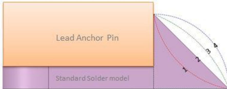
Figure 4-7 Profiles of varying solder mass
