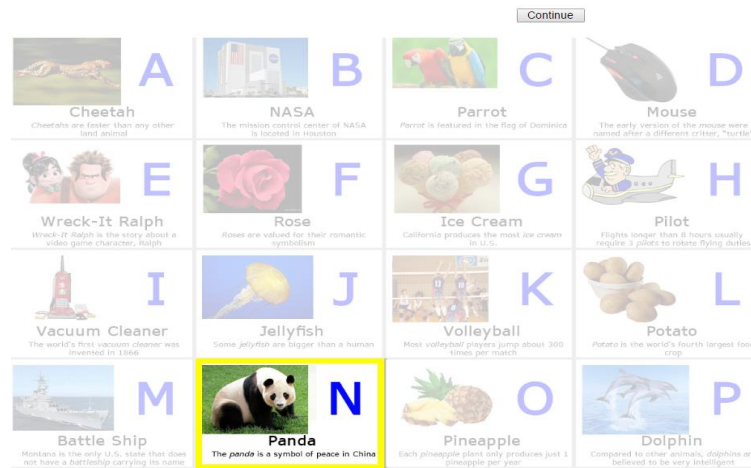
Fig 4.2 Registration Screen 2: The system-assigned keyword is highlighted, thus providing spatial cues about the keyword's location and the other objects nearby.
