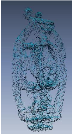
Figure 2-4: Point Cloud of Upright [4]
