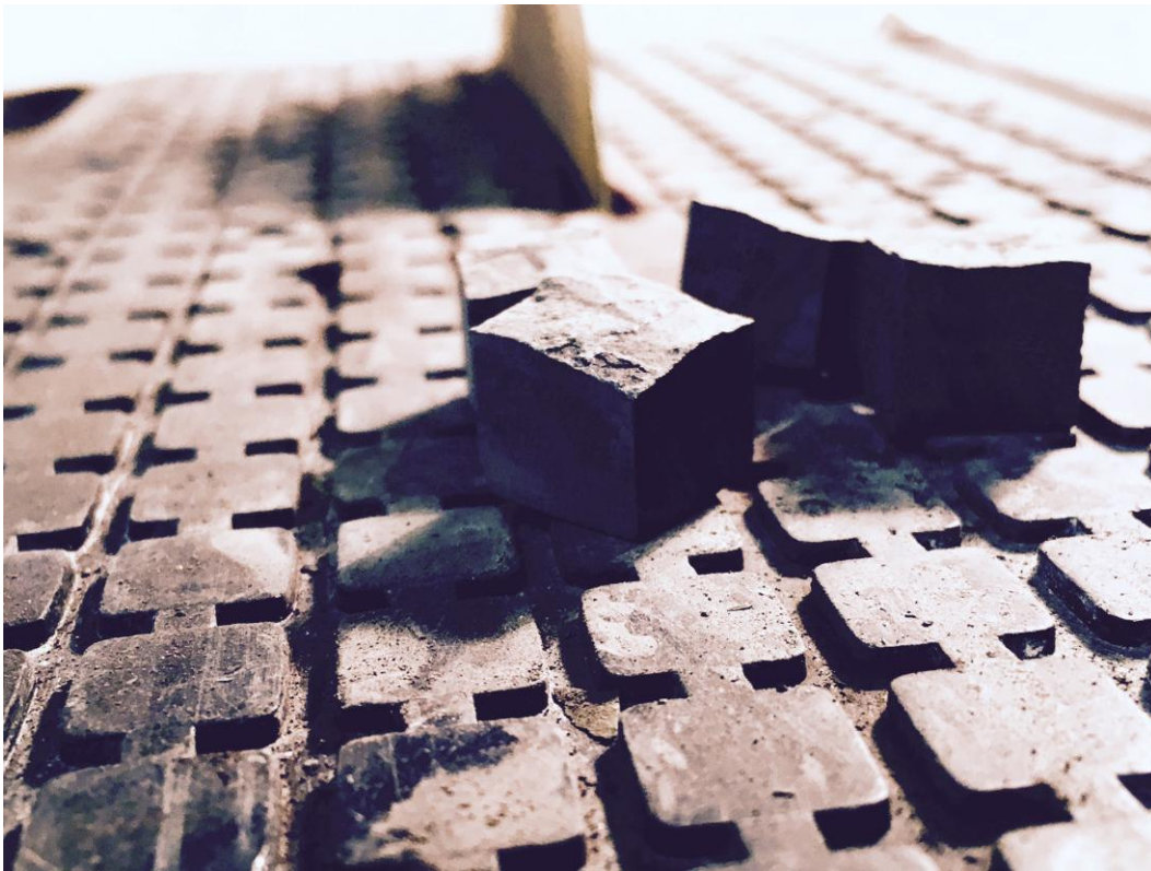
Figure 3-4: Sample Image of Cubes prepared for Imbibition.
