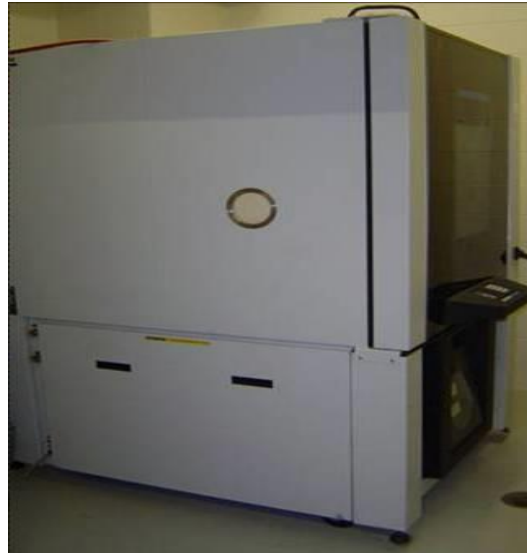
Fig 4: Thermotron Environmental Chamber SE600 10-10
