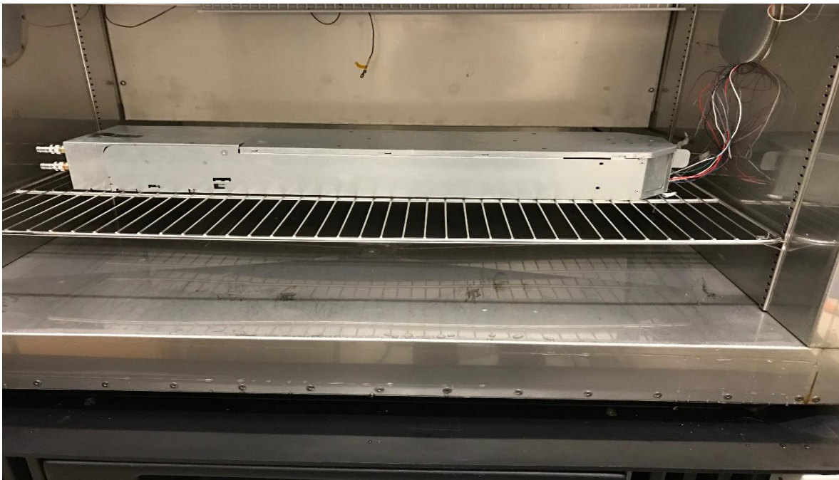
Fig 16: Open Compute Server Kept inside a Thermotron environmental chamber
