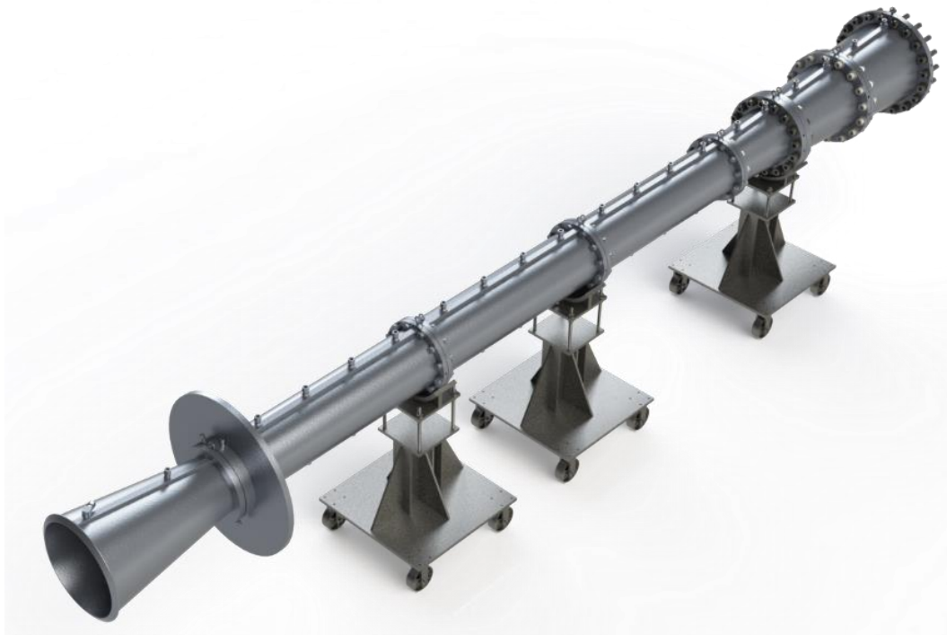
Figure 2.6: UT Arlington AHWT-II upgraded diffuser assembly.
