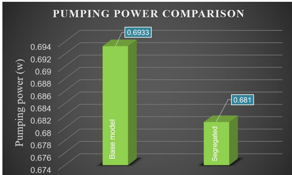
Figure 4-5 Pumping power of base and Segregated model at 1.3lpm flow rate
