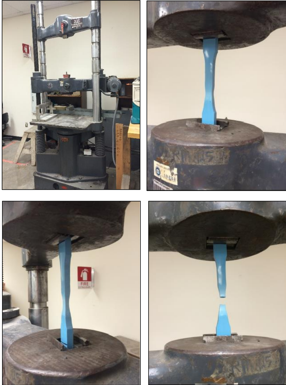
Figure 4-9 Tensile Test Type III (Full-wall) Testing at CUIRE
