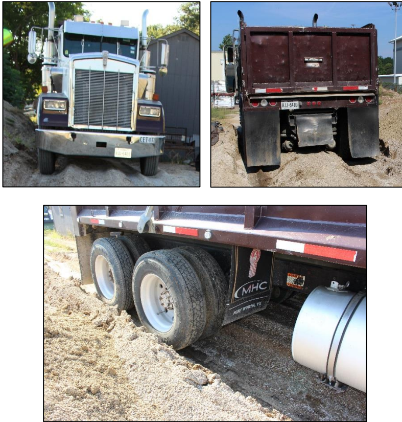
Figure 4-19 20-Ton Truck used to Create Live Load Simulation
