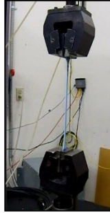
Figure 4-6 Type I Tensile Test (Mid-wall) in Action at Microbac
