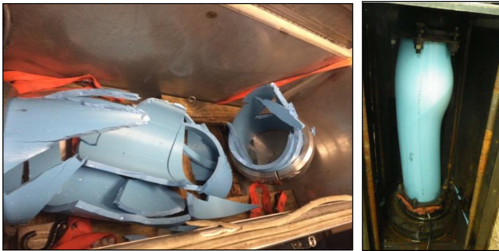
(a) (b) Figure 4-1 iPVC pipe Failure in Short-term Burst Pressure Test: (a) Brittle Failure and (b) Ductile Failure (Source: WRF Report No. 4650, 2016)
