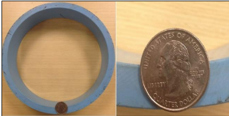
Figure 2-19 9 in. OD DR 18 iPVC pipe Thickness (Source: AW and PPI, 2015)
