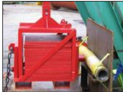
Figure 2-6 Full Scale Impact Test Setup (Gabet et al. 2011)
