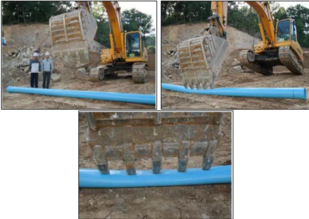
Figure 2-23 Bucket Test (Source: AW and PPI, 2015)
