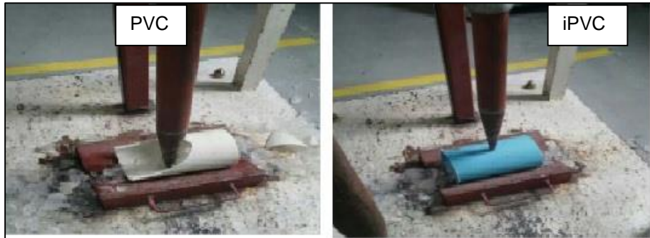
Figure 2-20 PVC and iPVC pipe Impact Test Results (Source: AW and PPI, 2015)
