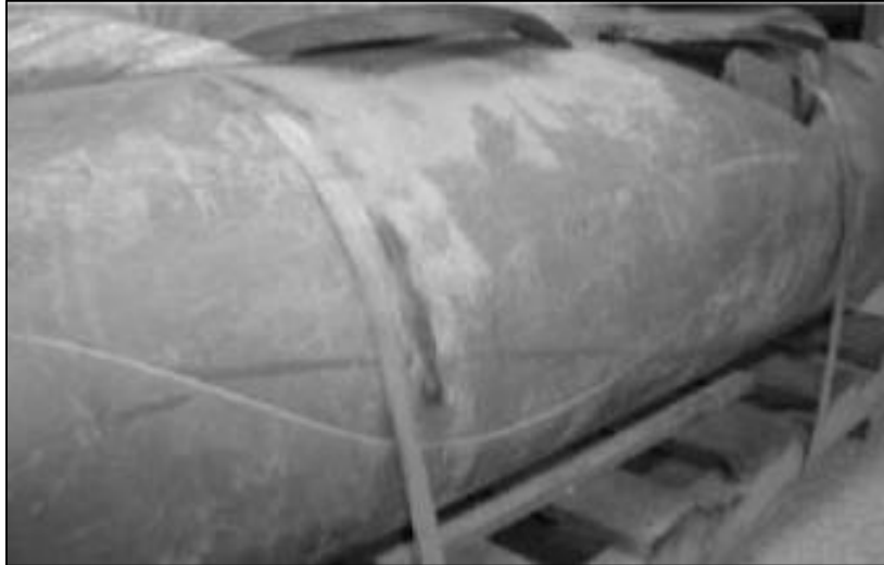
Figure 1-10 Crack in PVC Pipe (Burn et al., 2005)
