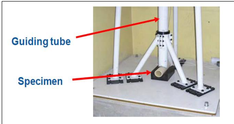
Figure 2-5 Small Scale Impact Test Setup (Gabet et al. 2011)
