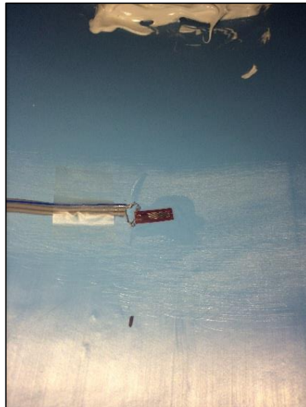
Figure 3-9 Strain Gauge attached to iPVC pipe
