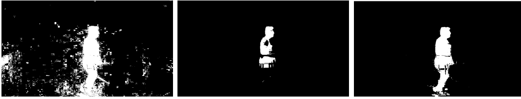
Figure 4.5: Figures from left to right represent the result of the filter for threshold values 10,100 and 30 respectively.
