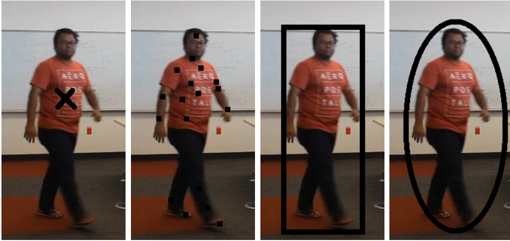
Figure 4.1: Figures from left to right represent various object representation (a) centroid, (b) set of points, (c) geometric shape - rectangle and (d) geometric shape - ellipse respectively
