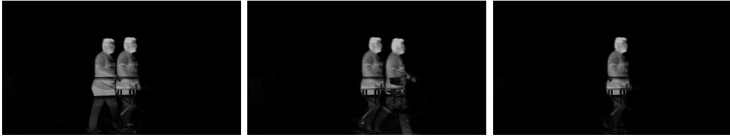
Figure 4.4: Figures from left to right represent the difference between frame 1030 and 1010, difference between frame 1030 and 1050 and motion of object in frame 1030 respectively.
