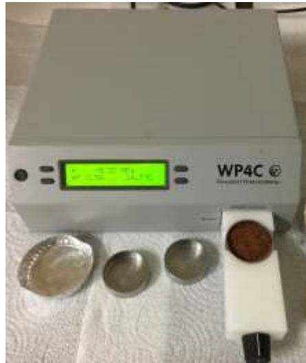
Figure 2.9 WP4 chilled water Potentiometer
