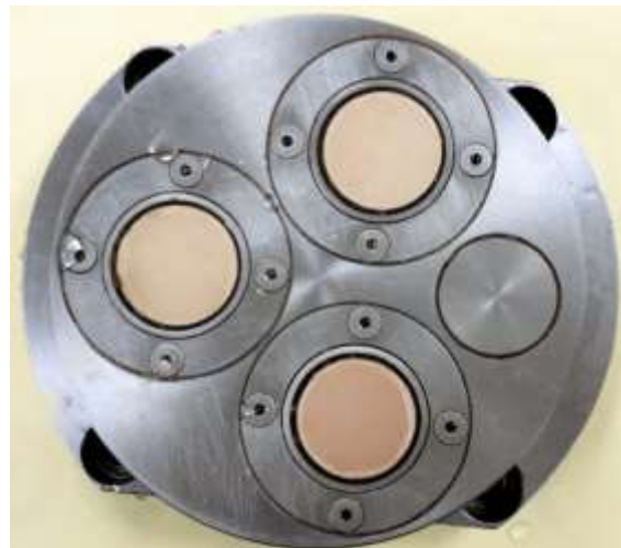
Figure 3.16 The assembled base pedestal fitted with ceramic disks
