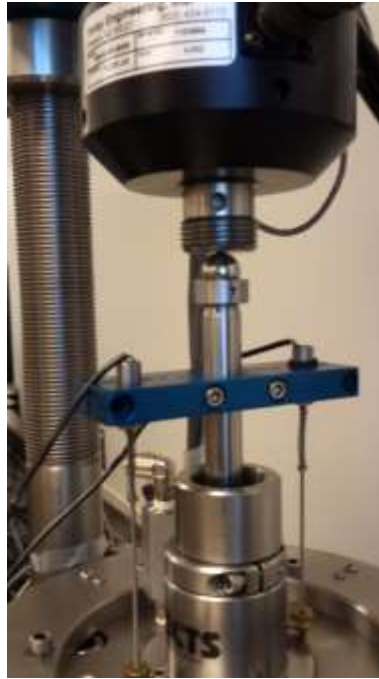
Figure 5.9 Modifications to the triaxial device for performing suction-controlled RLTTs
