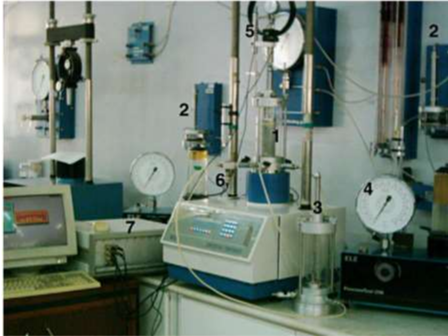
Figure 2.23 Modified triaxial testing equipment (Kayadelen, 2007)
