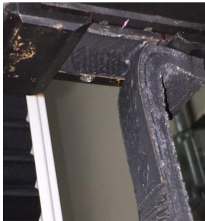
Figure 4-4 Adhesive Strength of elastomer
