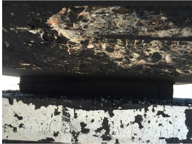
Figure 3-7 Bearing pad after fire test
