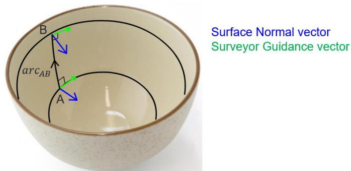
Figure 22 Occasion when the dot product is zero between the path vector and the SG vector
