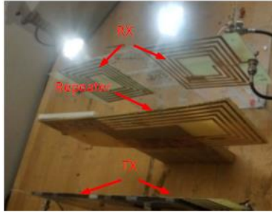
Figure 4-12 Demonstration of the prototype MIMO system. The system is able to deliver 5 W to each light bulb connected to RXs with an overall transfer efficiency of 80% at 5.83 MHz, 6.78 MHz and 8.48 MHz
