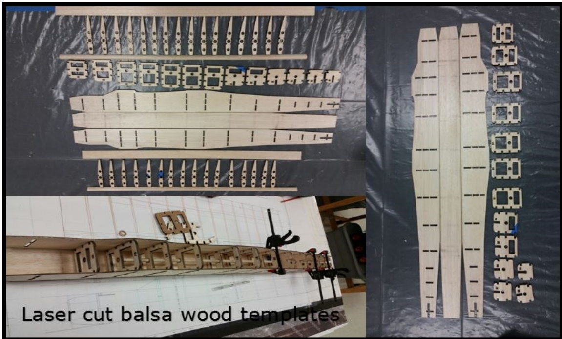
Figure 2.9. Laser cut balsa templates of whole aircraft.
