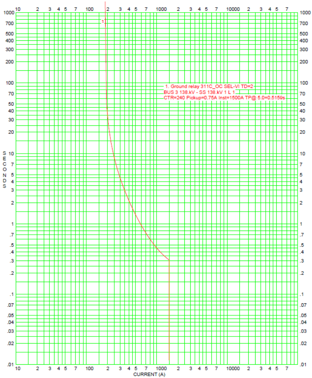
Figure 4-7 SEL421 Ground Overcurrent element Time Current Curve (TCC)
