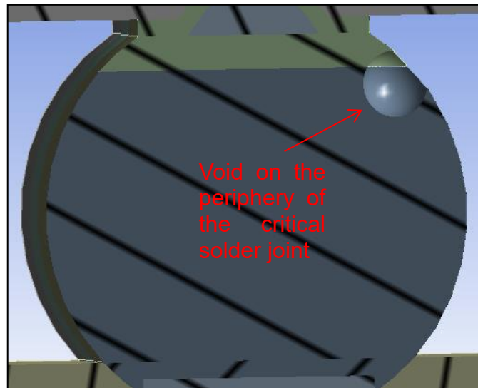
Figure 3- 3 Case I Void at the corner of critical solder joint
