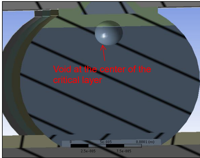
Figure 3- 4 Case II Macro void at the center of the critical layer
