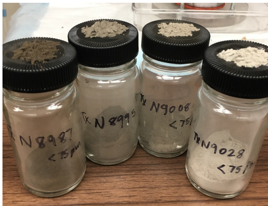
Figure 4-5 Powder fraction of <#200 mesh (<75 \mu\text{m} ).
