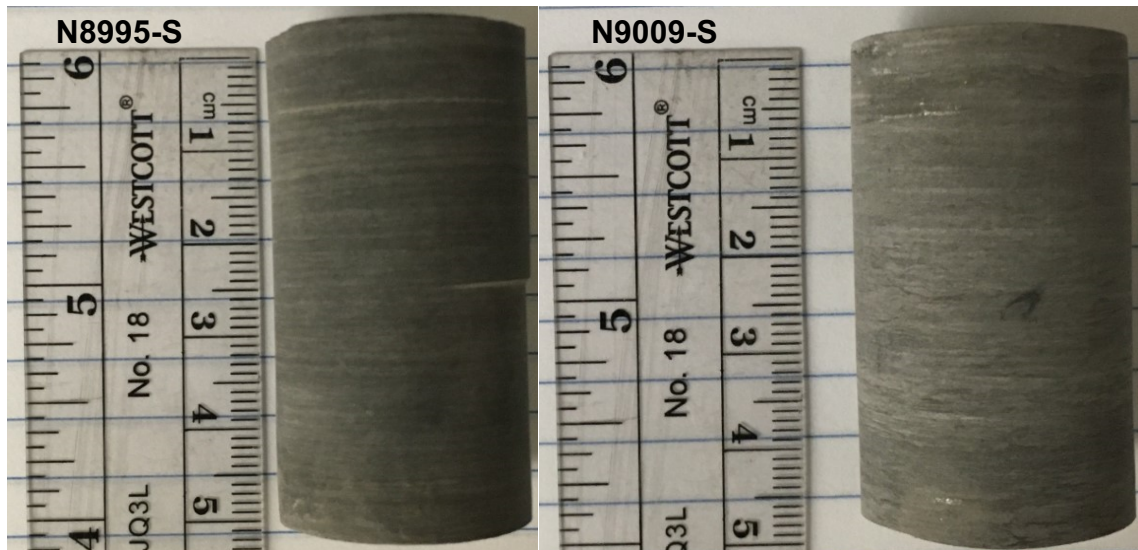
Figure 4-2 Core plug size fraction 1" x 2" taken from depths 8995 ft. and 9009 ft.
