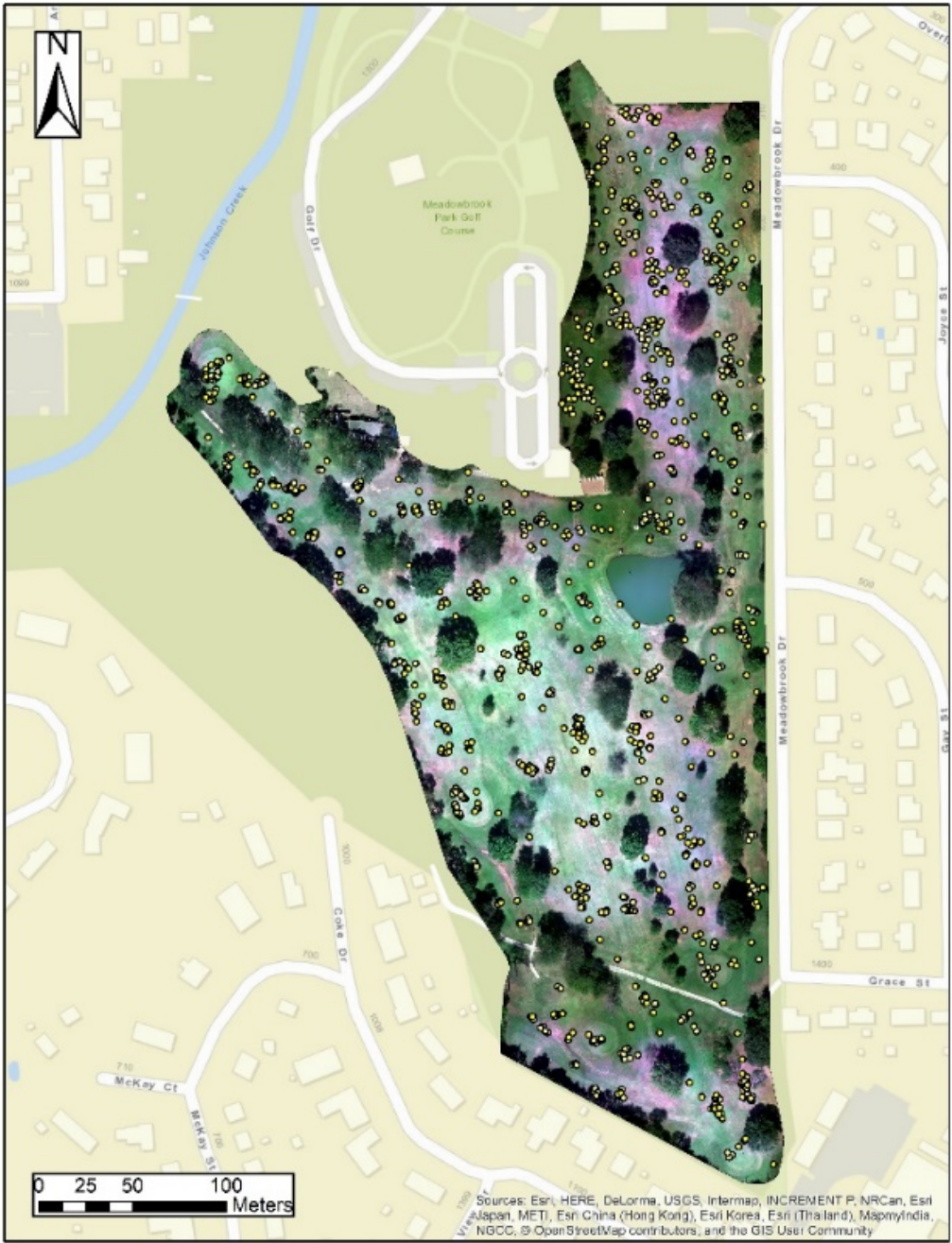
Figure 2-5 Spatial distribution of soil moisture samples from FieldScout TDR 300.
