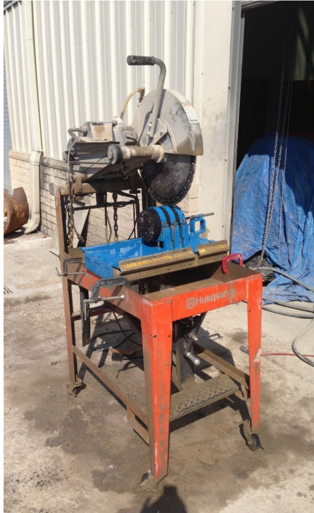
Figure 4-4 Setting up the Wet Saw Machine
