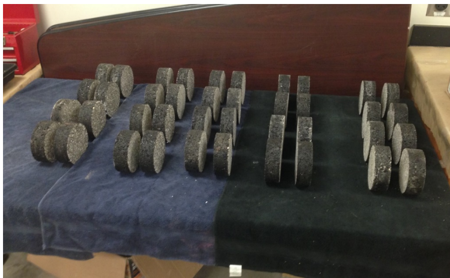
Figure 4-6 Specimens in Pairs after Cutting
