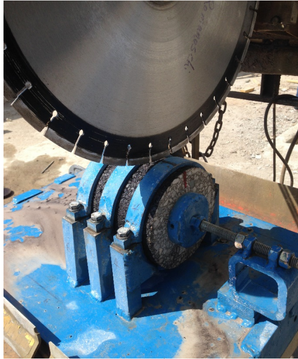
Figure 4-5 Marking and Adjusting the Sample Position for cutting
