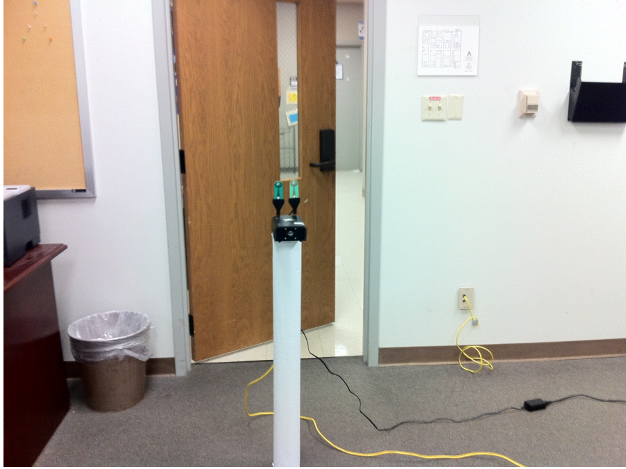
Figure 5.7. Location of the UWB radar on another side of a Wooden Door.
