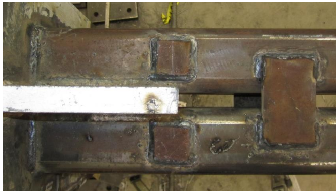
Figure 4-24 Top view of SP 5 shows cover plates and horizontal stitches.
