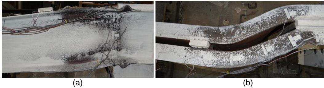
Figure 4-10 (a) Side view and (b) front view of 2C12-9 at 0.088 member rotation
