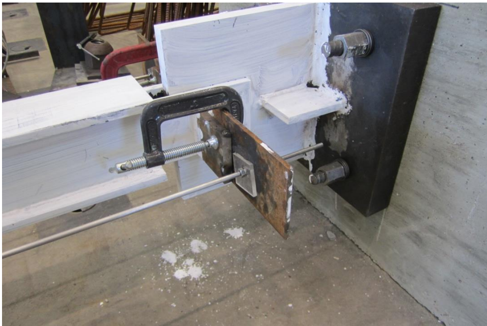
Figure B-9 LVDT Extension Connecting to the Other End of the Specimen, 3 rd Trial
