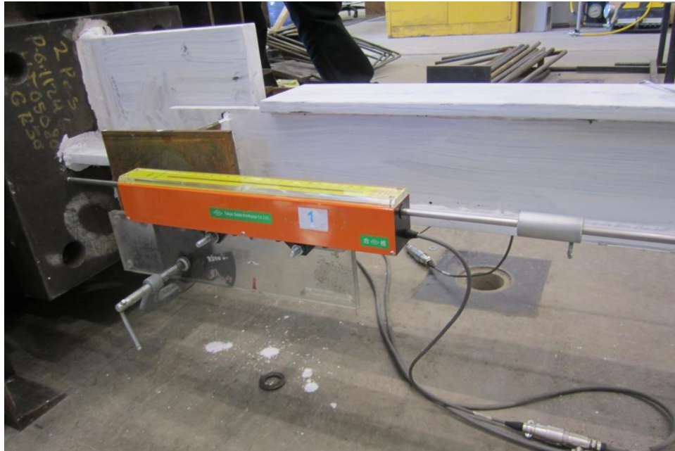
Figure B-8 Connection between LVDT and Specimen, 3 rd Trial
