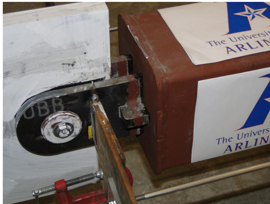
Figure 4-35 Elongation of the Steel Core on the East End
