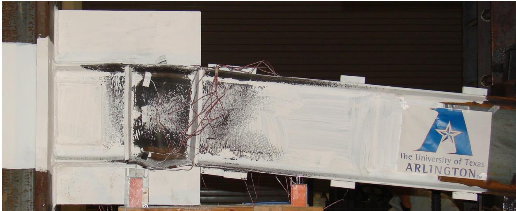
Figure 4-3 Specimen 2C12-3 at 0.028 rad STMF Story Drift
