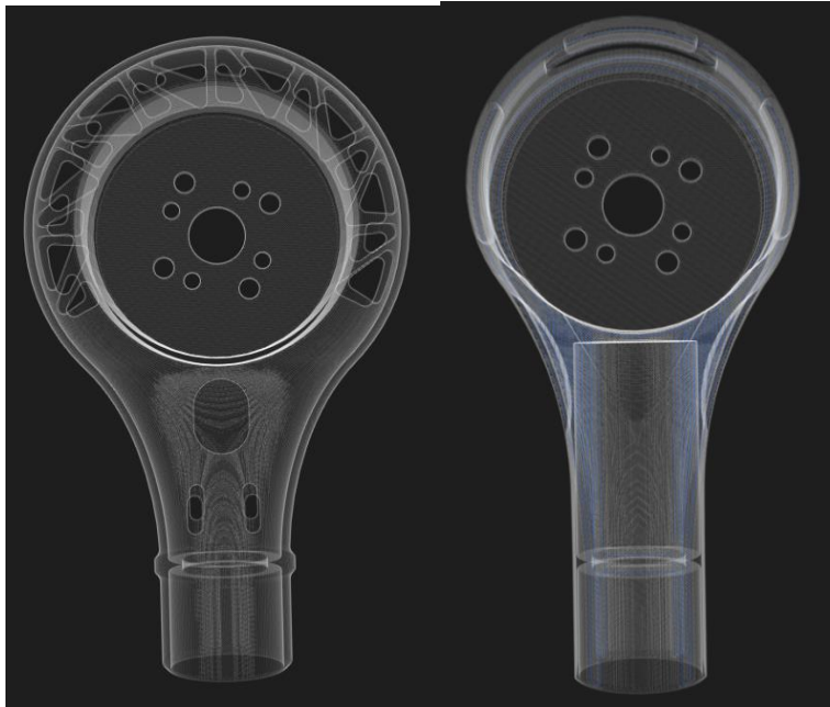
Figure A5: Original motor mount (Left) and redesigned Motor Mount (Right) (Eiger)
