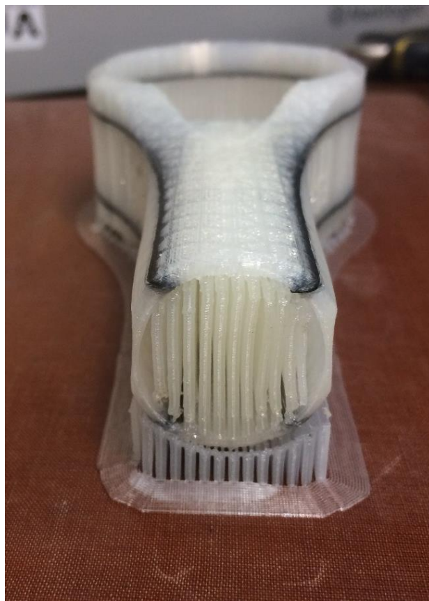
Figure B8: Completed part with support material
