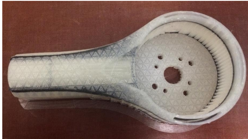
Figure B7: Completed part with support material
