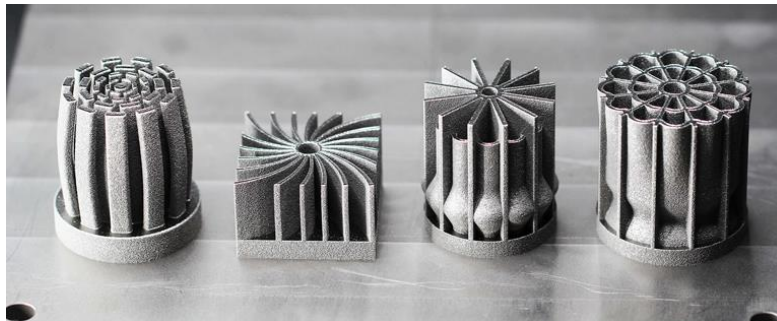
Figure 2-3 Heat sink Designs Created using a metal 3D printer [10]
