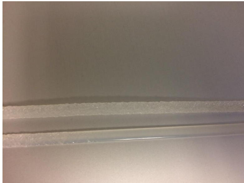
Figure 2-2 Wet nylon (top) vs dry nylon (bottom)
