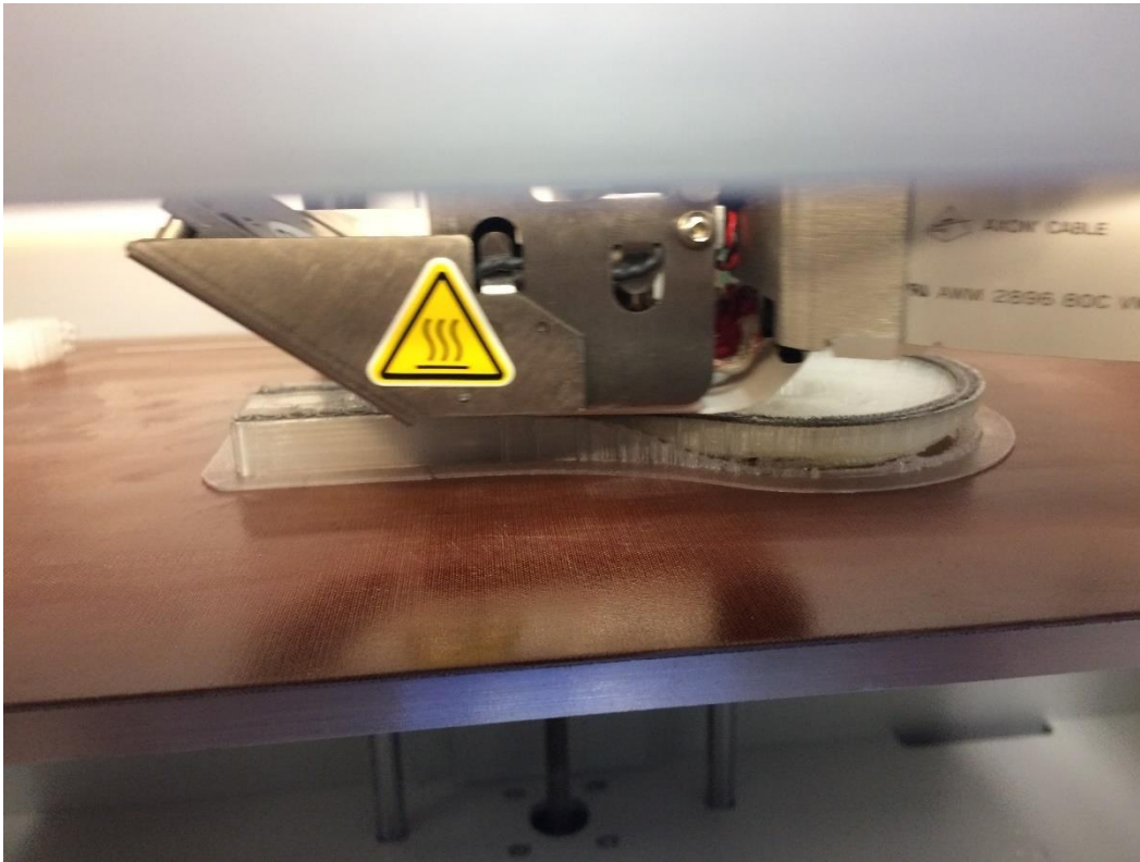
Figure 3-1 Printing a carbon fiber layer
